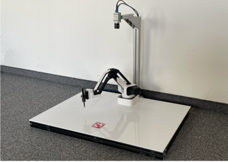
Figure 5.10: Affordable robotic manipulator Rotrics DexAm used for deployment of the proposed model-based contact detection approach.
