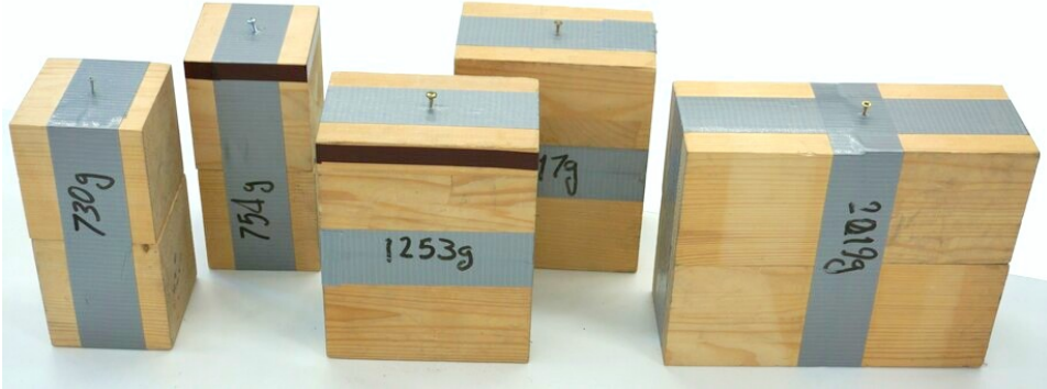
Figure 6.2: The set of weights used in the experimental evaluation of acting wrench estimation.
