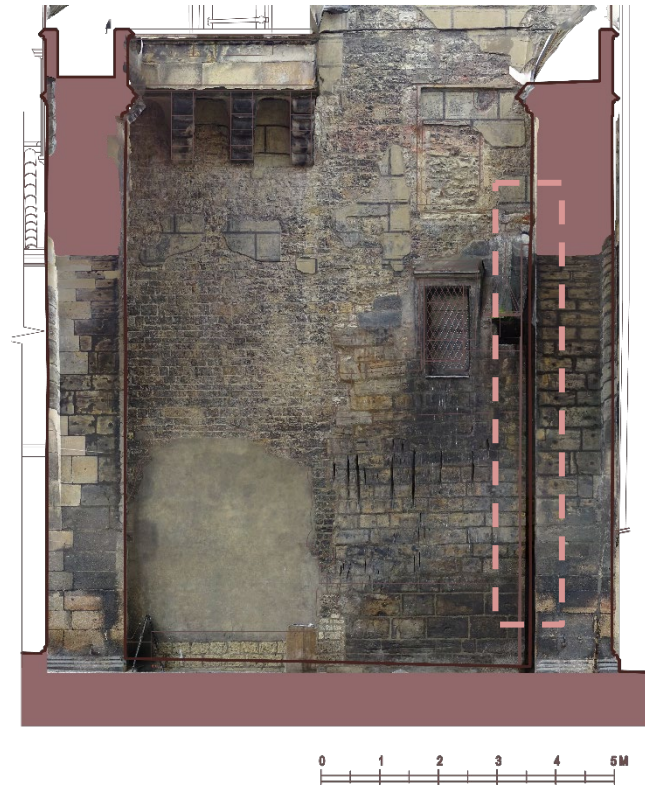
Figure 4.3 The lower part of the Northern façade, the dashed line highlighted the vertical groove.
