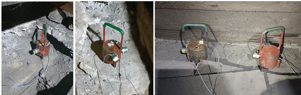
Figure 5.16 Second setup - accelerometer placement
