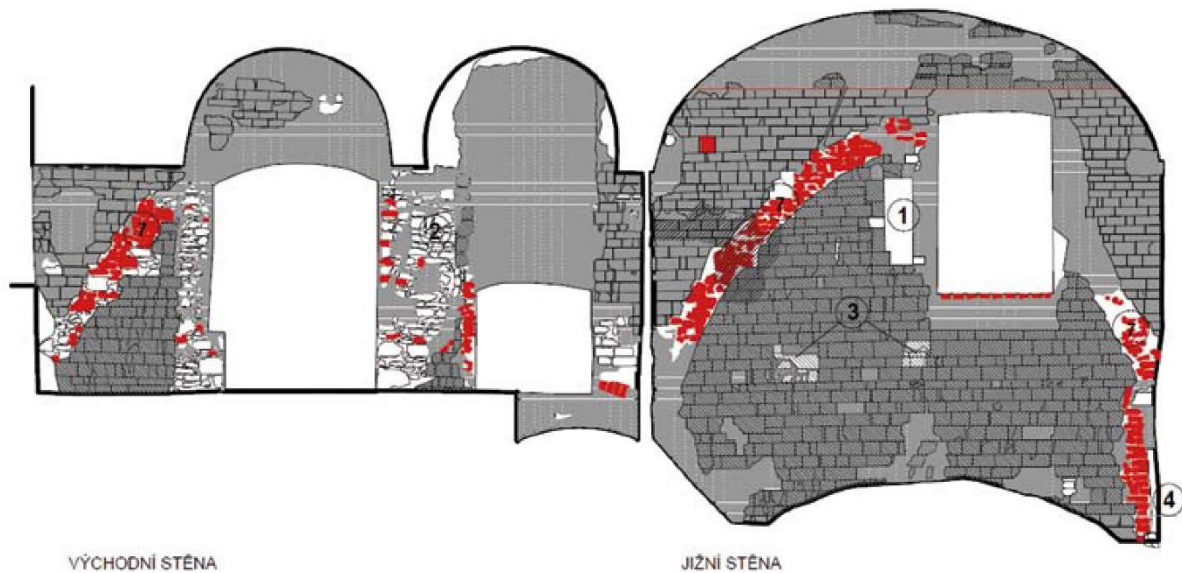
Figure 3.6 Detailed survey and documentation of the ground floor walls, with an evaluation of findings processed by Jan Veselý, 2005-07.
