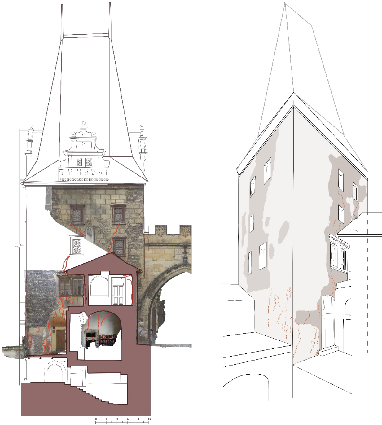
Figure 4.5 Eastern façade – (a) orthoimage documentation of the damaged part of the facades, (b) sketch showing the façade deficiencies and damages.
