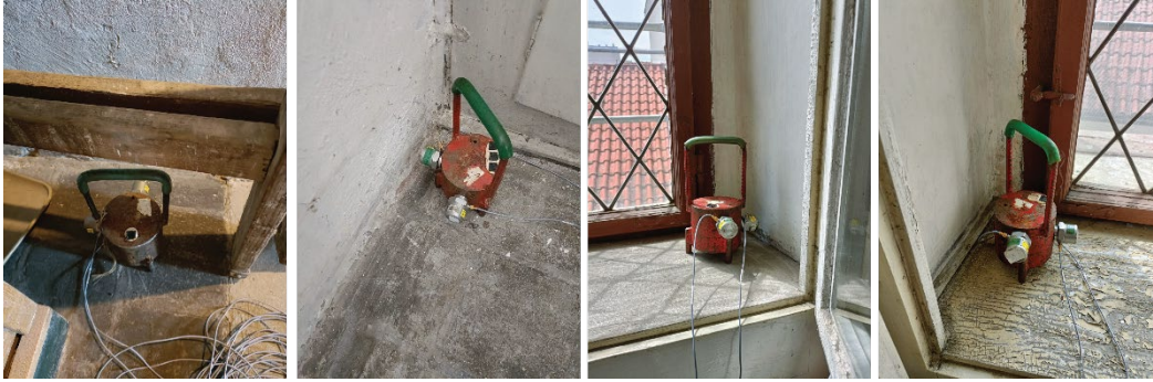
Figure 5.15 First Setup - accelerometer placement
