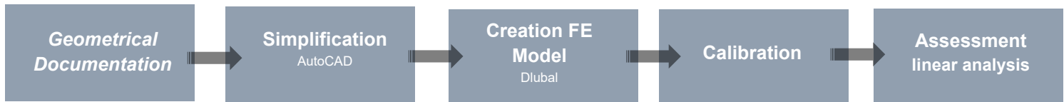
Figure 5.1 Creation of the Finite Elements Model – Methodology
