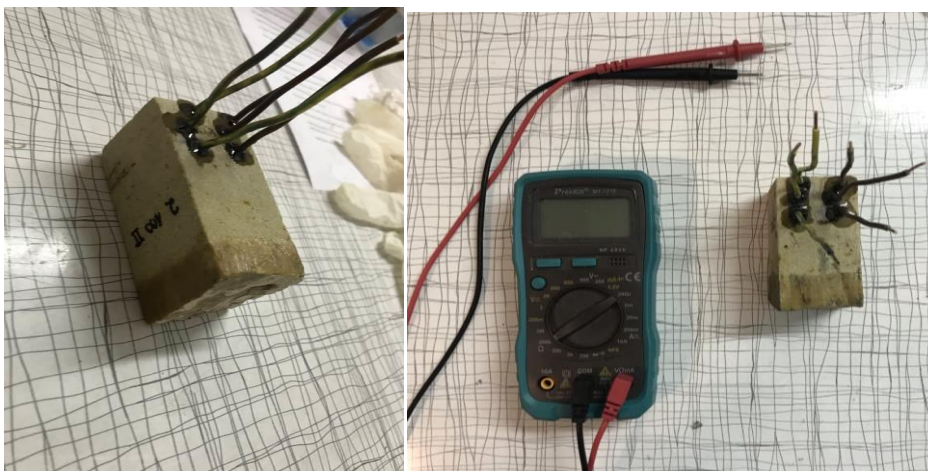
Figure 14: Left-Clean specimen. Right-Check to prevent the measurement from being influenced by surface resistance values.
