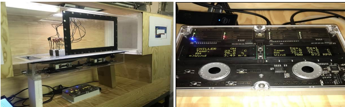
Figure 17: Samples in the wind tunnel and assignment of wind speed, temperature and relative humidity parameters.
