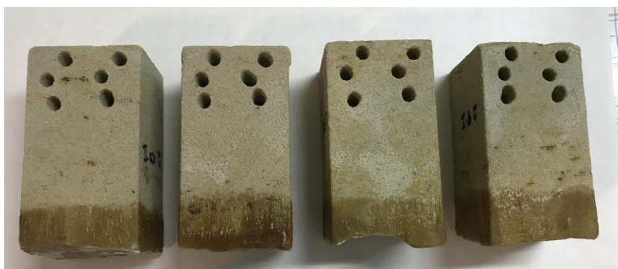
Figure 12: Drilling in the sample for electrode installation
