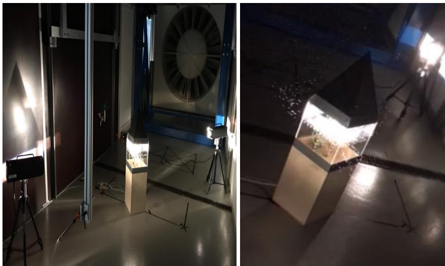
Figure 31: General test setup with tower at 45 degrees.
