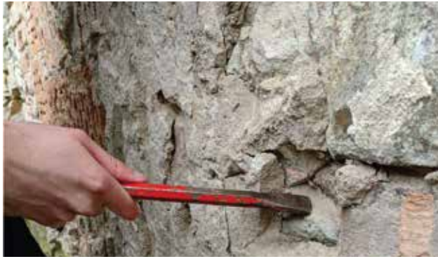
Fig 26: Sampling stone with chiesel.
