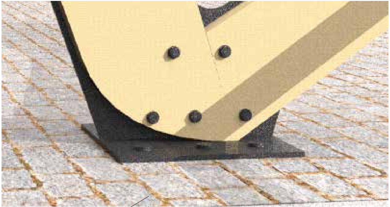
Fig 67 .The metallic plate inserted within the timber members is screwed outside with metallic bolts Leaving an offset of 5 cm outline outside of the timber members
