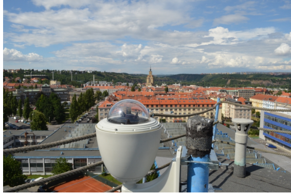
Figure 2.13: The WILLIAM all-sky ground-based imaging and monitoring system. Adopted from [A.1].
