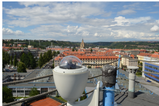
Figure 1. The WILLIAM all-sky ground-based imaging and monitoring system.
