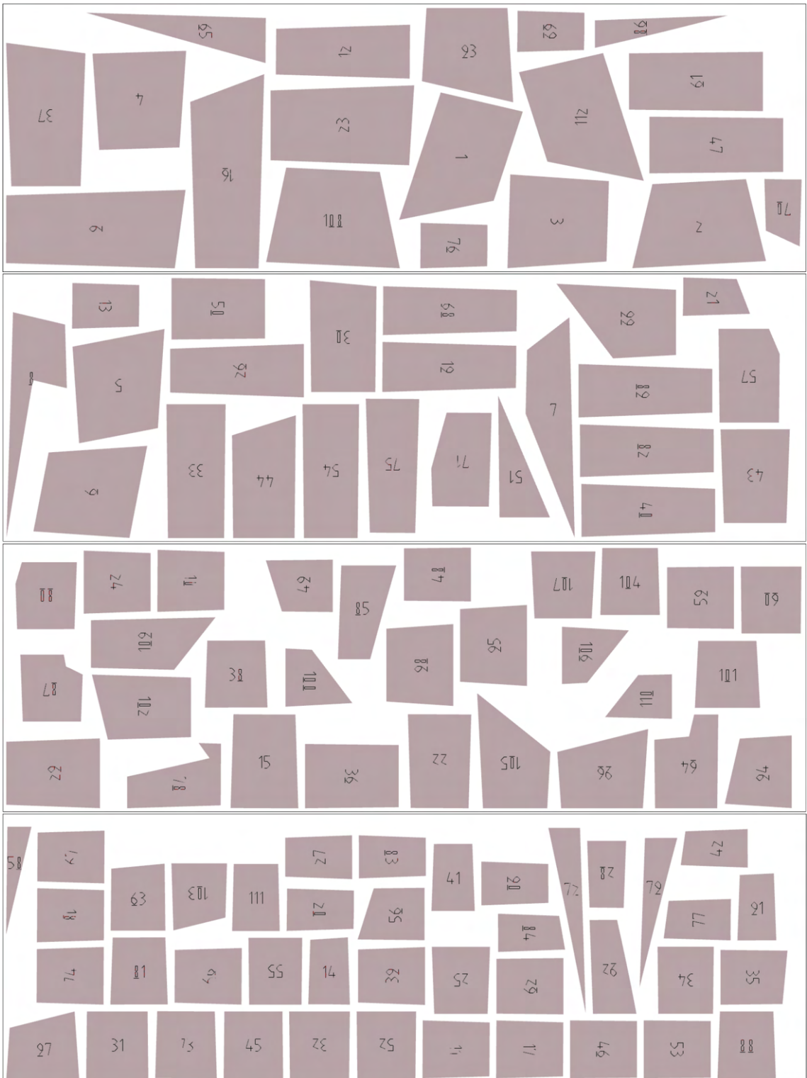
Figure 20: Generated formwork with small pieces
