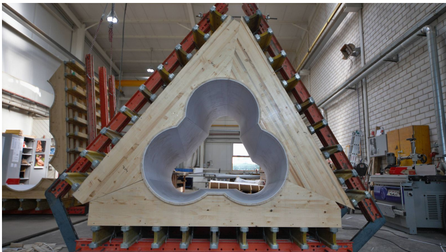
Figure 9.9: Showcase of a column formwork with a finishing plastic layer on sheathing [18]
