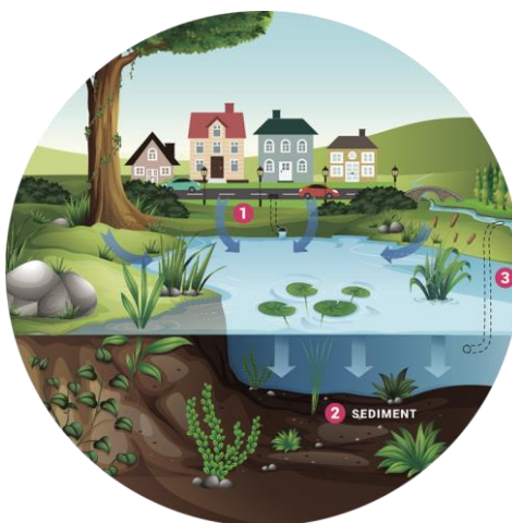
Obrázek 34 - Princip sedimentačního rybníku, zdroj: https://www.hamilton.ca/home-neighbourhood/water-wastewater-stormwater/stormwater-management/stormwater-management-ponds
