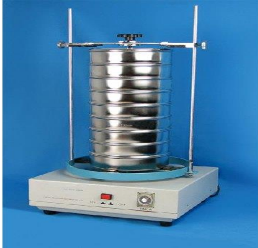
Fig.22: sieve shaker machine picture [from https://www.indiamart.com/proddetail/sieve-shaker-machine-12947348948.html ]
