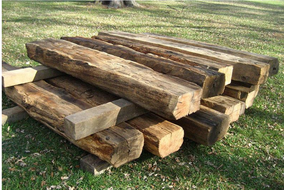
Fig.15: Reclaimed lumber [ from http://yr-architecture.com/reclaimed-timber-benefits-and-challenges/ ]
