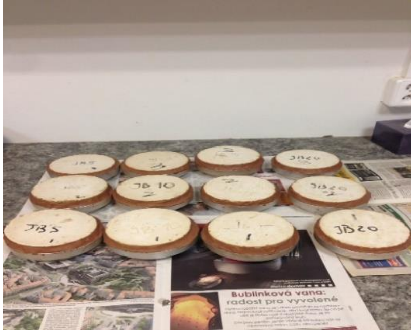
Fig. 24. Dry cup with silica gel
