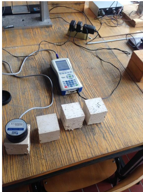
Fig. 25. Isomet 2114 in process of measurement
