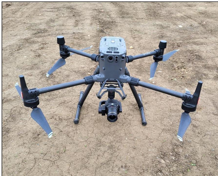
Obr. 10: UAV DJI Matrice 300 RTK s kamerou DJI Zenmuse P1
