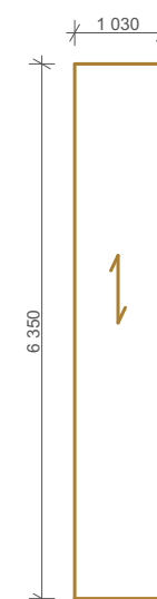
O.1 Novatop OPEN 227 mm (SWP 27 + KVS 60 x 200)
