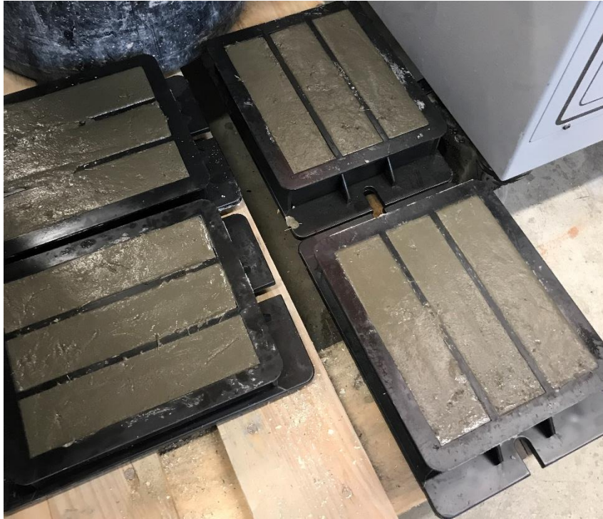
Figure 9 - Set of 12 beam samples in the forms – reference mixture HPC_REF
