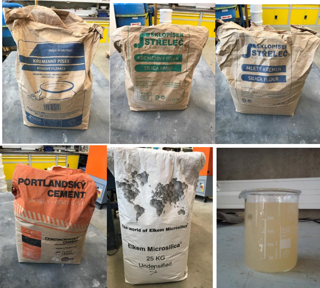
Figure 4 - Materials used in the HPC mixtures - different fractions of natural aggregate, cement, silica fume and superplasticizer
