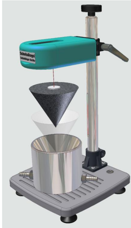
Figure 16 - Shrinkage measuring cone device
