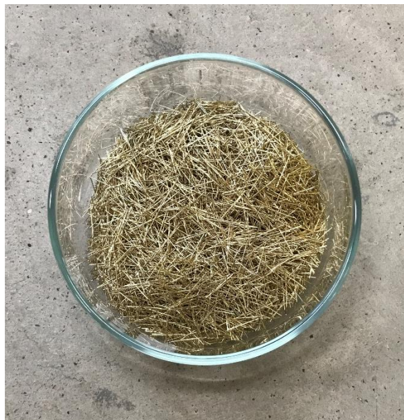
Figure 5 - All the samples contained steel fibers
