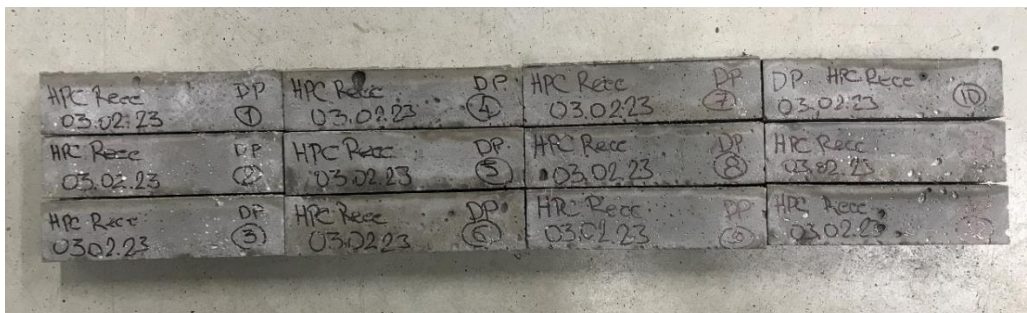
Figure 10 - Set of 12 beam samples all made from one mixture – HPC_3
