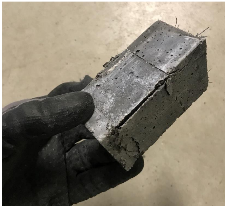
Figure 15 - Broken sample after the compressive strength test
