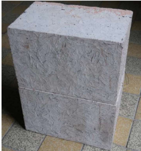
Figure 5 Tested specimen, material U after thermal conductivity measurements (at the TZ laboratory).
