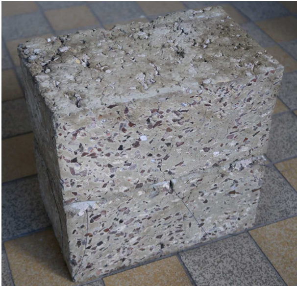
Fig. 6. Tested sample, material S after thermal conductivity measurements (at the TZ laboratory).
