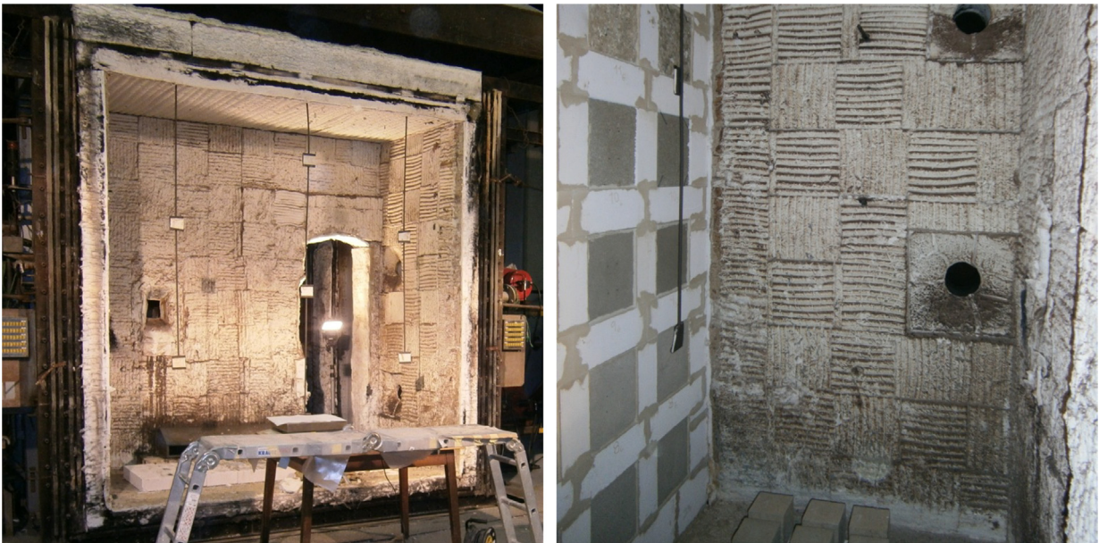
Fig. 3. A vertical furnace used for the fire test: the furnace without the test wall (left); inside view of the furnace with the test wall and the test specimens set in place (right), see also [24].
