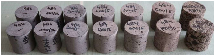
Figure 10 Tested samples after the permeability test, material U.
