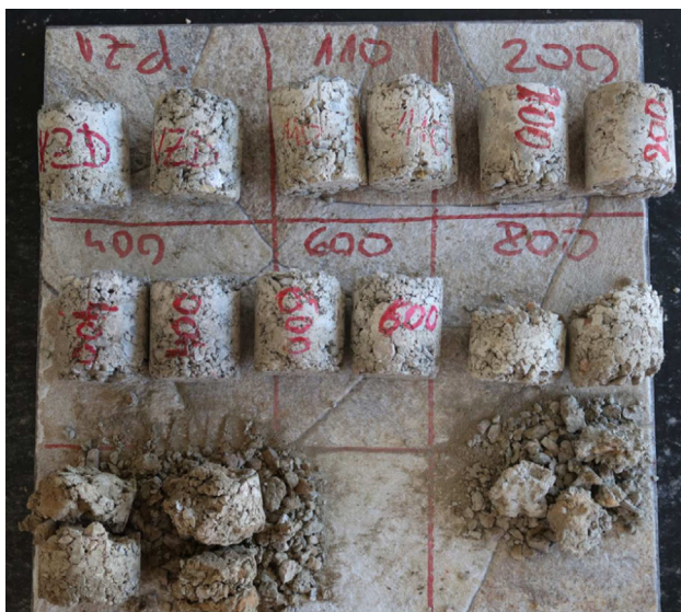
Fig. 11. Tested samples after permeability test, material S.
