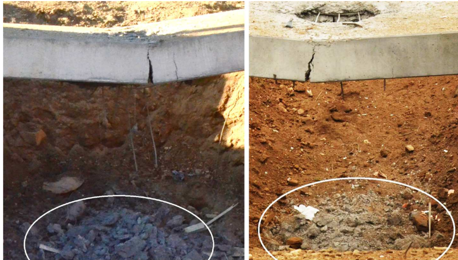
Fig. 24. A comparison of the amount and the size of the fragments after the blast for specimen no. 18 (left image) and for specimen no. 19 (right image).
