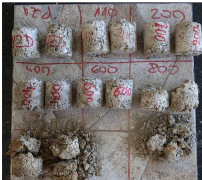
Figure 11 Tested samples after permeability test, material S.
