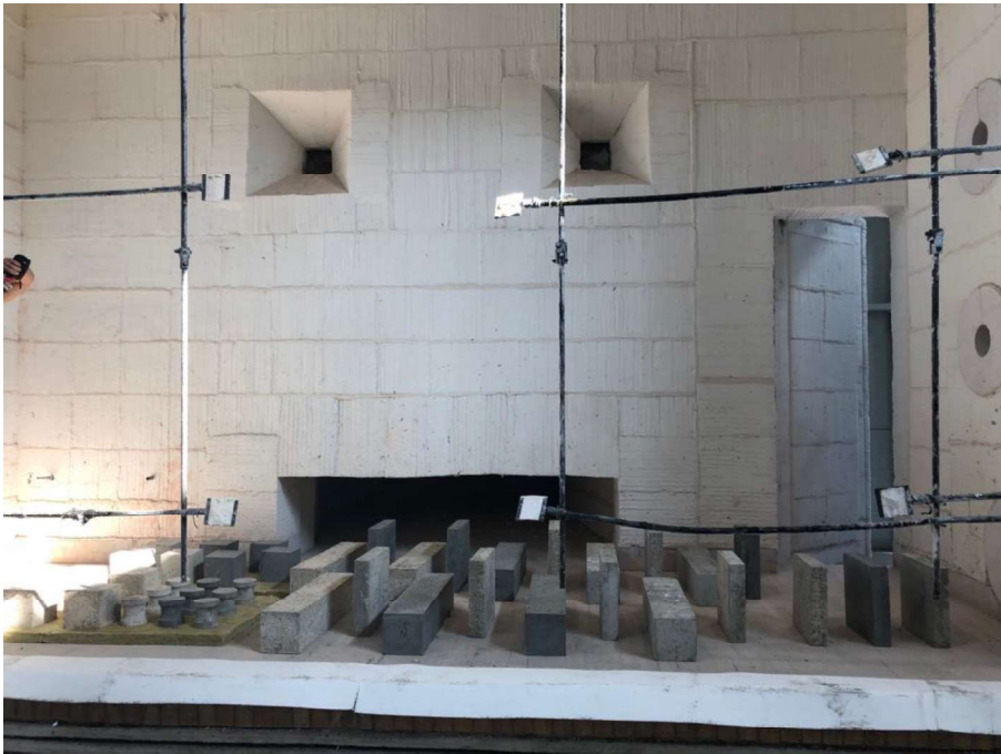
Figure 15 Arrangement of the specimens on the test furnace floor (view in the opened furnace)
