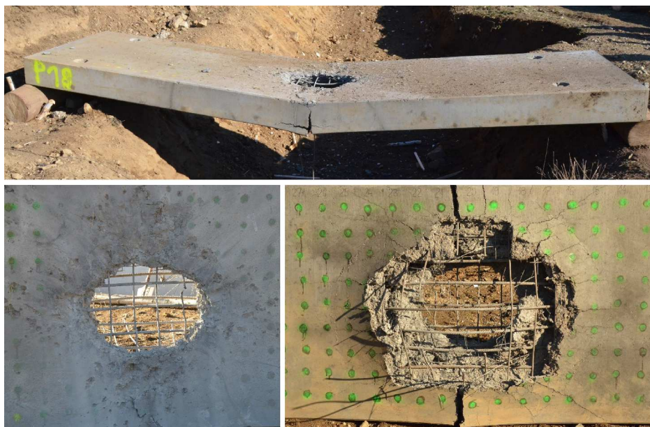
Fig. 17. Damage to specimen No. 18 after the blast. Overall view (top image), top view (bottom left image), bottom view (bottom right image).
