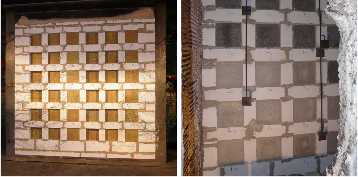
Fig. 5. Test wall with the wall-panel specimens: the outside view – the unheated surface (left); the inside view – the heated surface (right), see also [24].
