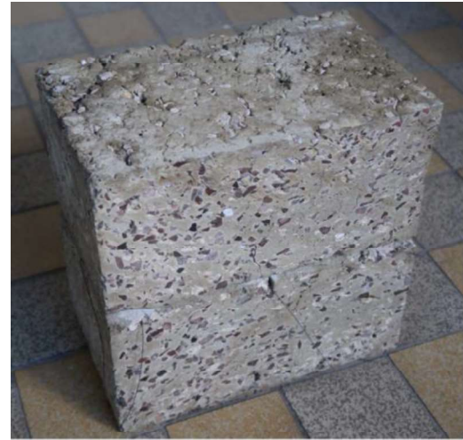
Figure 6 Tested specimen, material S after thermal conductivity measurements (at the TZ laboratory).
