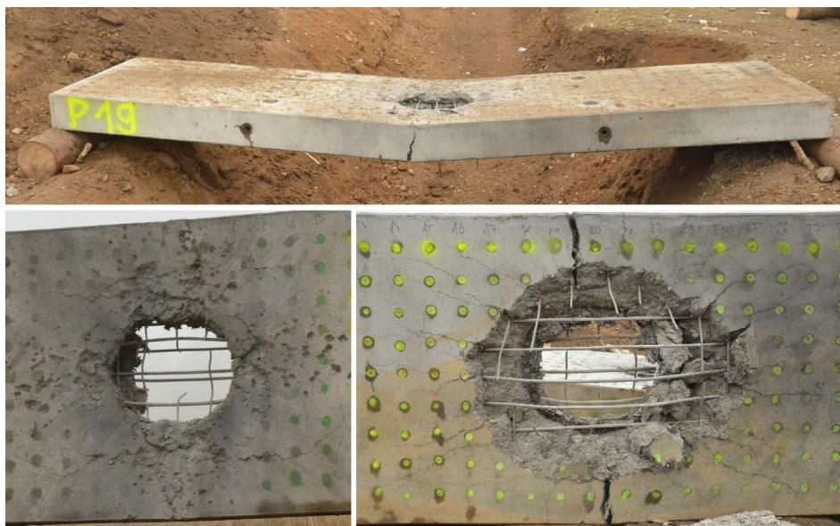
Fig. 23. Damage to specimen No. 19 after the blast. Overall view (top image), top view (bottom left image), bottom view (bottom right image).
