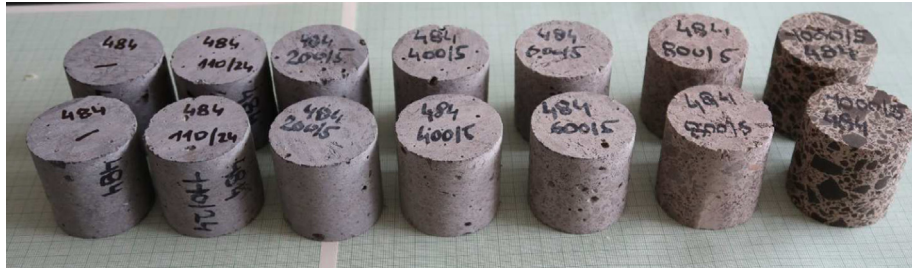
Fig. 10. Tested samples after the permeability test, material U.
