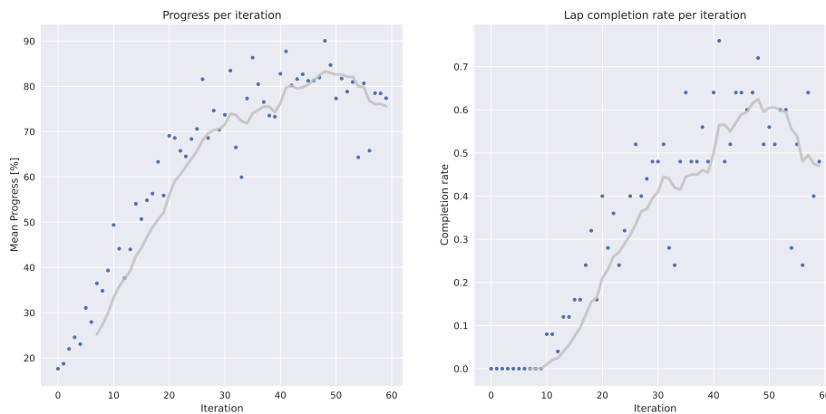
■ Figure 4.7 Mean iteration progress (left) and lap completion rate (right) for the 3-layer CNN model in an environment with moving obstacles.
