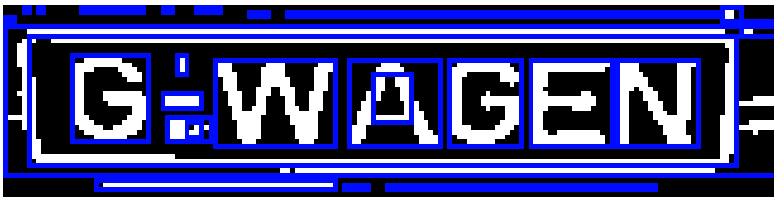
■ Figure 5.7 All detected contours on binarized number plate
