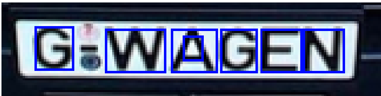
■ Figure 5.8 Filtered contours on color number plate
