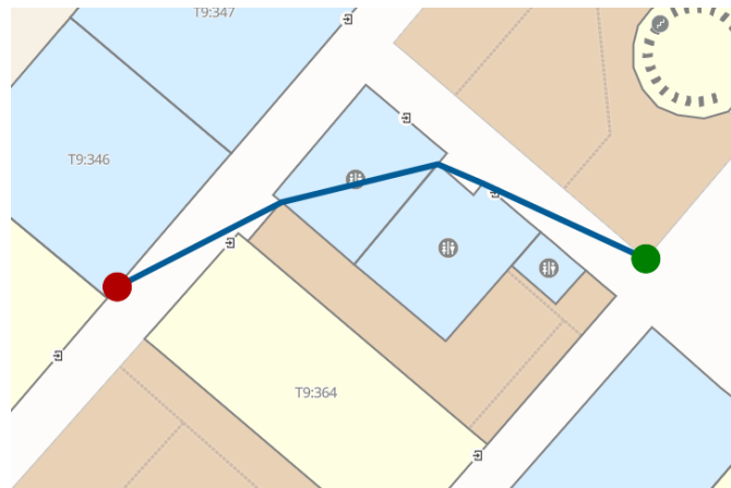
■ Figure 4.1 A bug where the application suggests a route through a wall.
