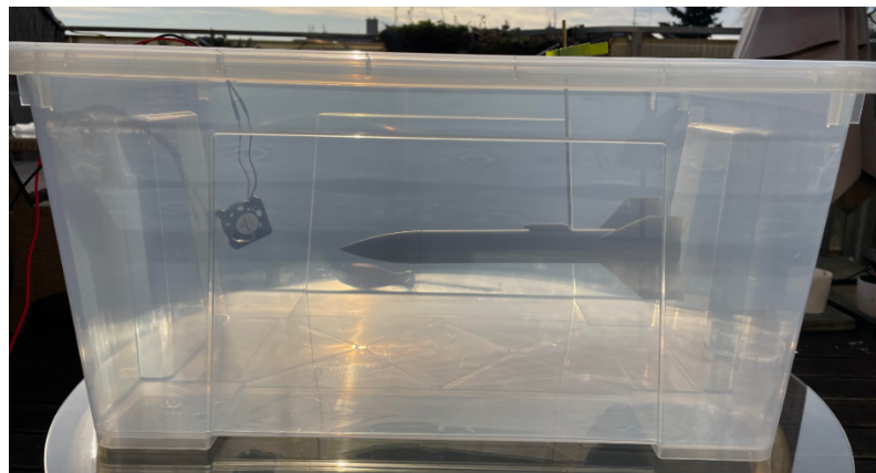
Figure 26 - Plastic PET container with an ASA rocket being treated with acetone vapor.
