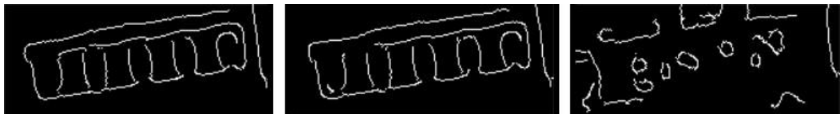
Figure 45 - edges of one detected cyclonic dial on three channels
