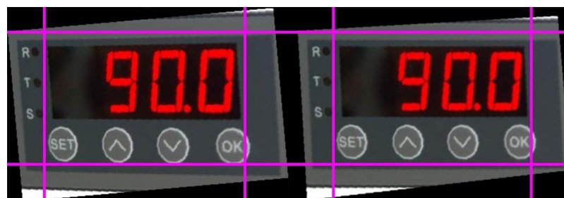
Figure 38 - A comparison of a warped image (right) with a rotated-only image (left) [34]
