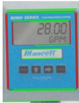
Figure 9 - A flow monitor with a segment display with detected lines by the lu_vp_detection algorithm [32]
