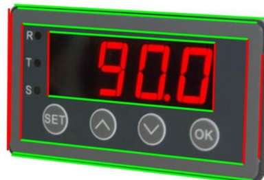
Figure 36 - Detected image with added context with lines detected by the lu_vp_detect algorithm [34]
