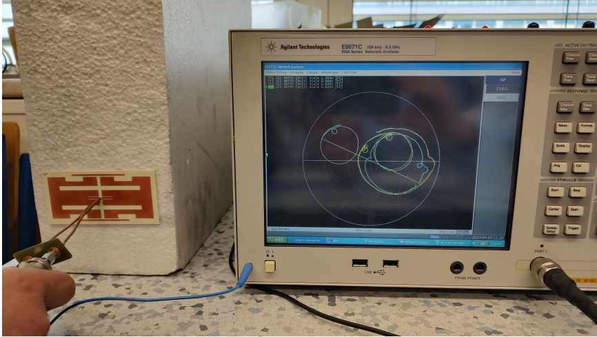
Figure 3.5: Measurement of antenna impedance. On the left: a differential probe from [6] is used. On the right: measurement is seen on a Smith chart. Note that a glitch is causing erroneous 180° phase shift which is later corrected in MATLAB.
