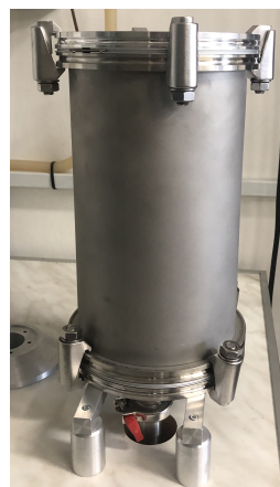
Figure 6.6: The sealed heating chamber. The vacuum pumps are connected by a bellow from the bottom.
