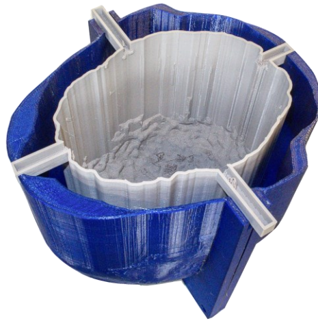
Figure 16: 3D printed molds for manufacturing of the 3D solid head phantom. Precise positioning of the inner mold in the outer mold, due to stabilizing stops, which also follow the exact pressing depth of the inner mold.
