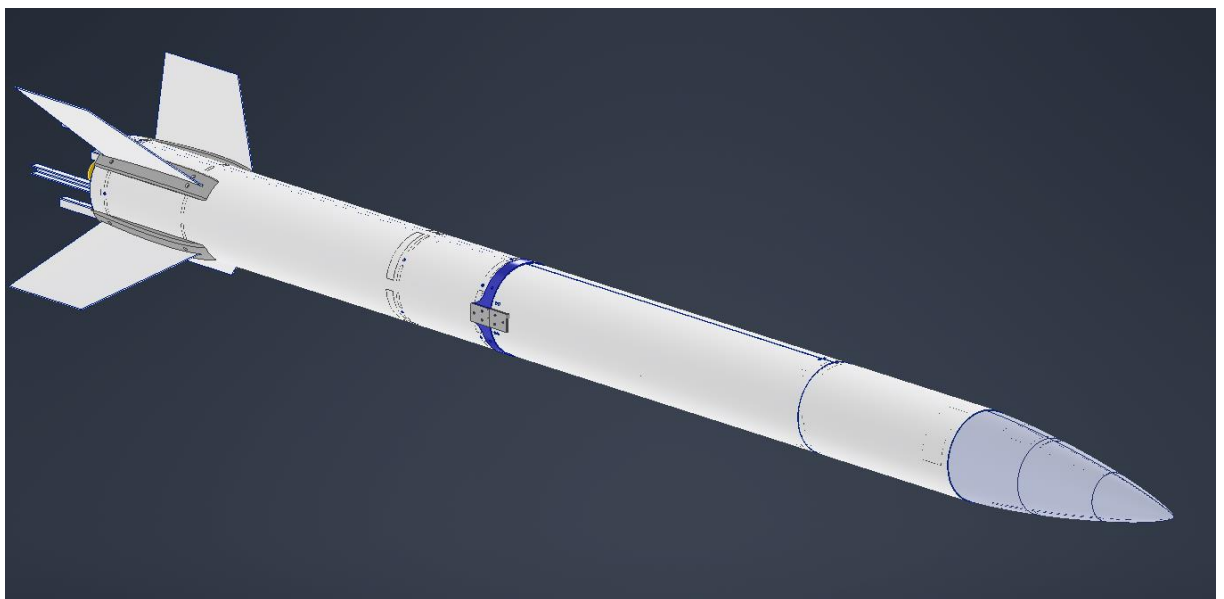
Obr. 14 - Sestava rakety Sherpa v programu Autodesk Inventor 2022
