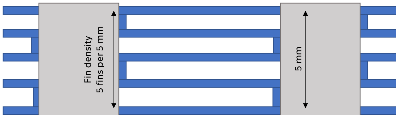
Figure 7-1: Representation of fin density within one fin row between 2 coolant tubes. The coolant tube surface is grey, and the fins are blue.
