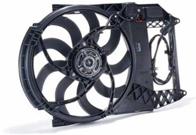
Figure 4-10: Electrical fan with a shroud which helps to distribute the fan-induced airflow across the radiator surface. [14]
