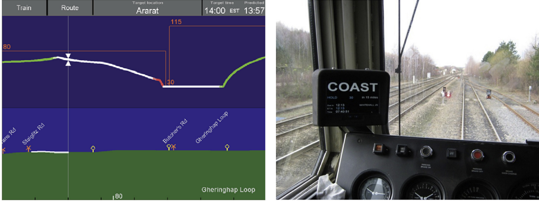
Figure 1.1: A photograph of the active Energymiser DAS. The system notifies the train operator when the control mode should be changed and also shows how long the current mode should remain active. The image is from Albrecht et al. (2015).
