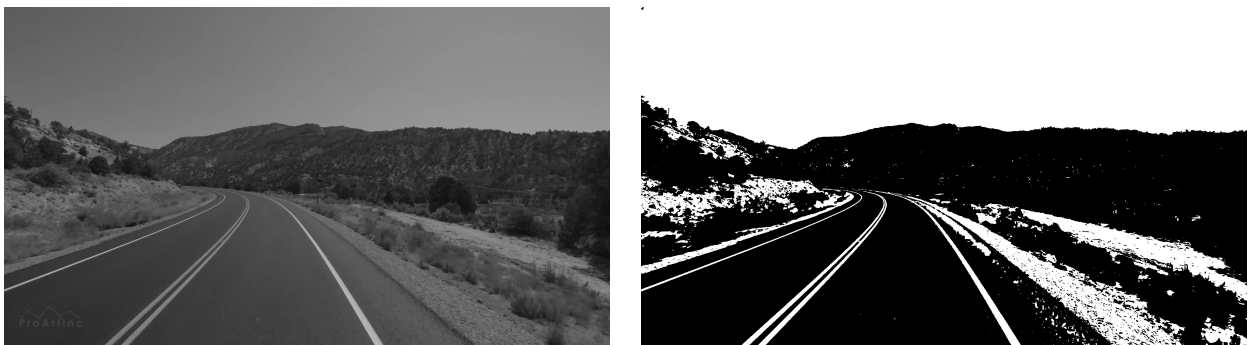
Figure 1.5: (a) Gray image; (b) Otsu applied to (a)
