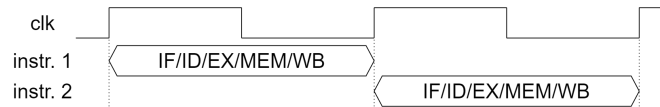
■ Figure 2.2 Instruction cycle of a single-cycle scalar microarchitecture. An entire instruction is processed in one cycle.
