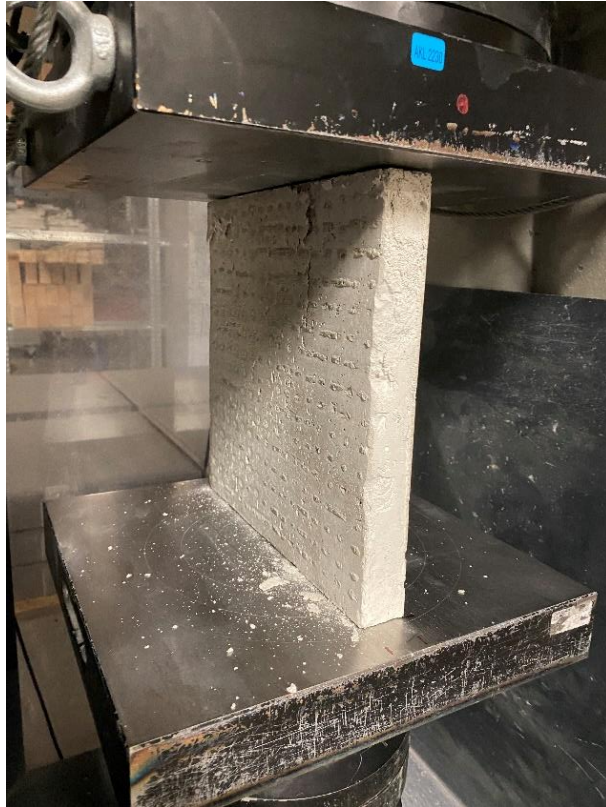
Figure 82: Compressive Strength Test – Solid slab with GF
