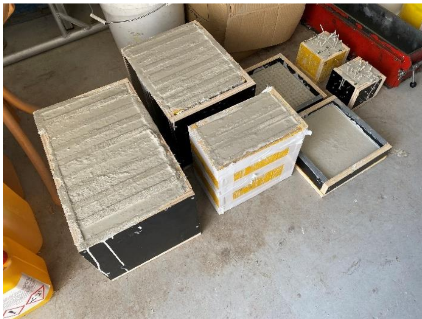
Figure 51: Formworks for making samples
