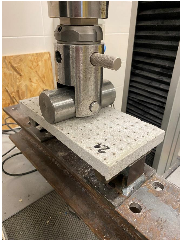
Figure 129: Tensile Flexural Strength Test - Slab with Air holes and GF – Sample 21
