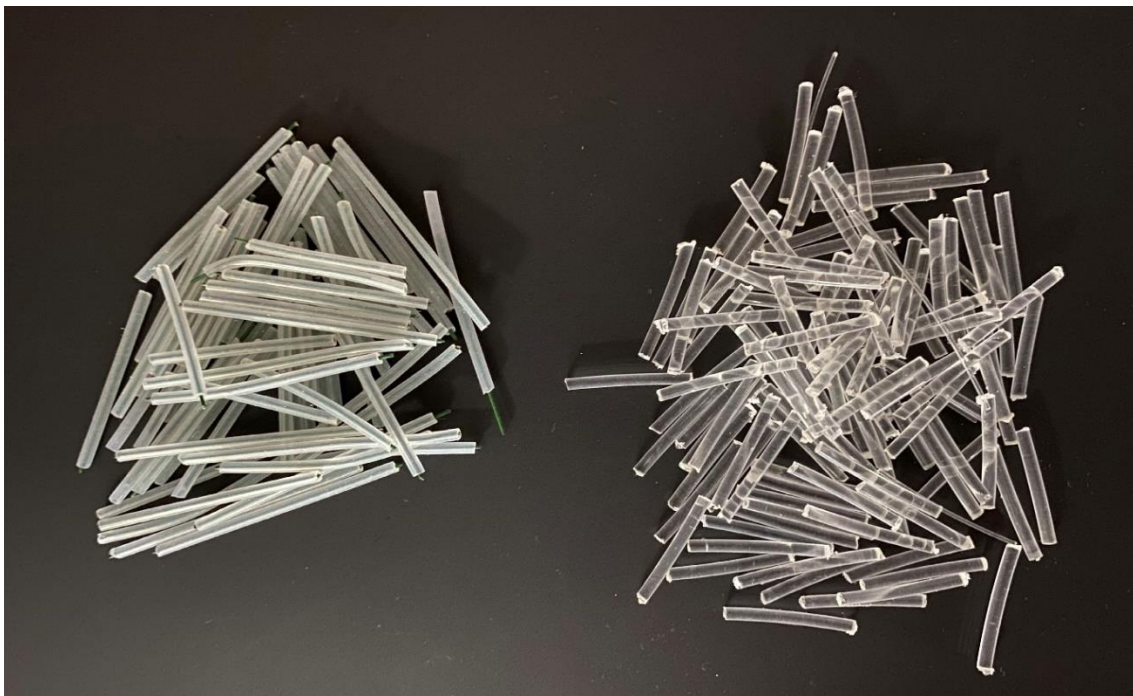
Figure 56: Plastic tubes with wires and optical fibers POF used for experiment
