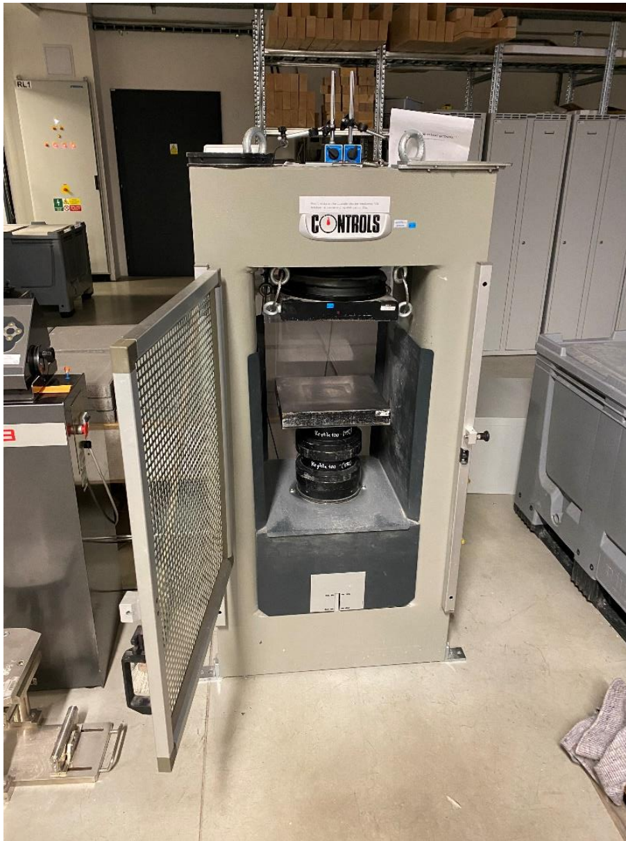
Figure 78: Compressive strength measuring machine – Controls C68Z00
