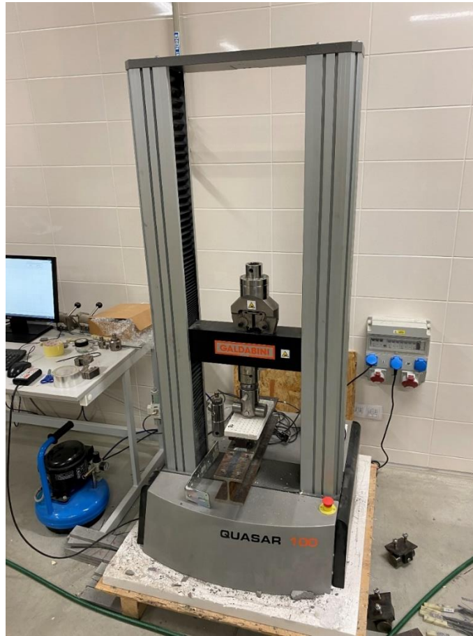
Figure 98: Tensile Flexural Strength Measuring Machine - Galdabini Quasar 100
