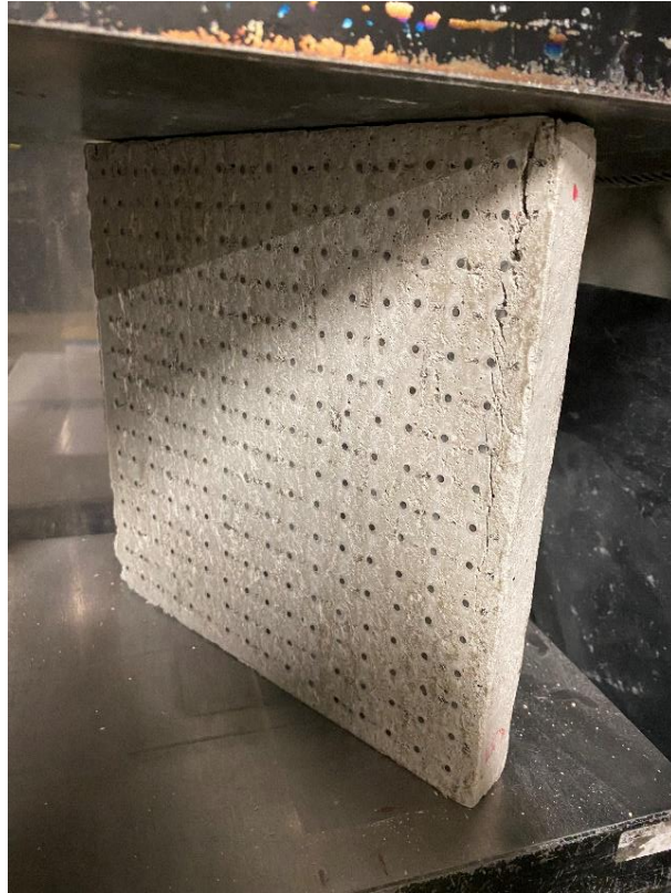
Figure 88: Compressive Strength Test – Slab with POF and GF
