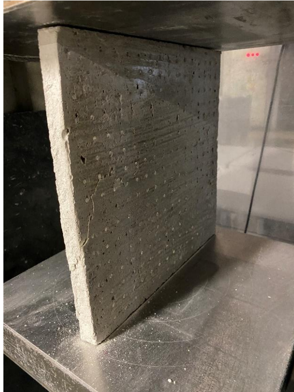
Figure 92: Compressive Strength Test – Slab with POF and GF
