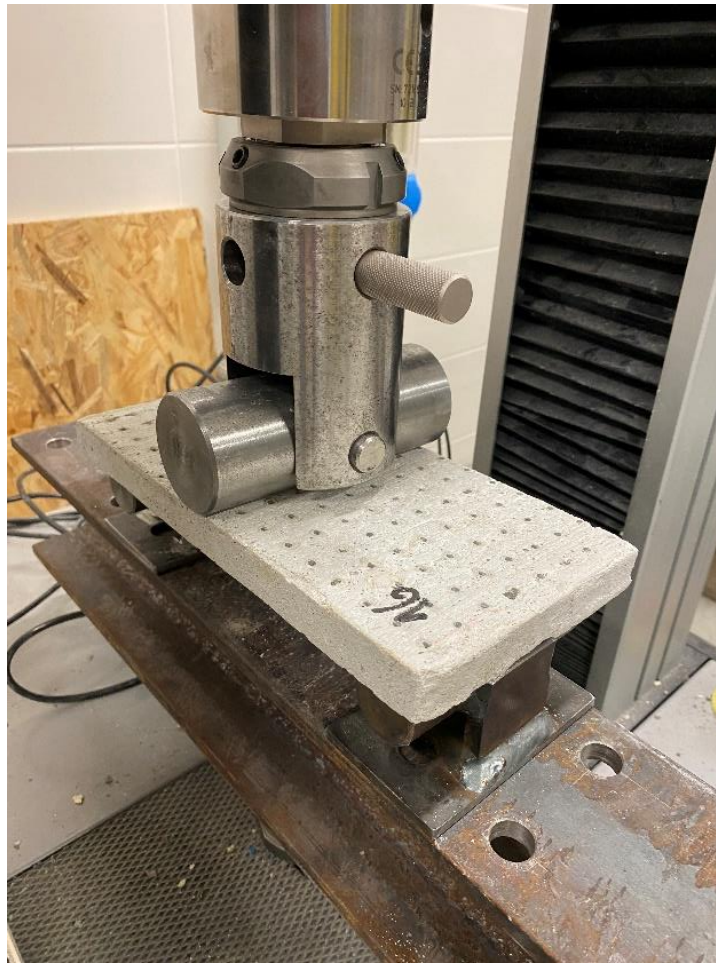
Figure 119: Tensile Flexural Strength Test - Slab with POF and GF – Sample 16
