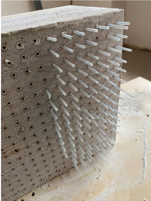
Figure 54: Sample with air holes, created by plastic tubes with wires
