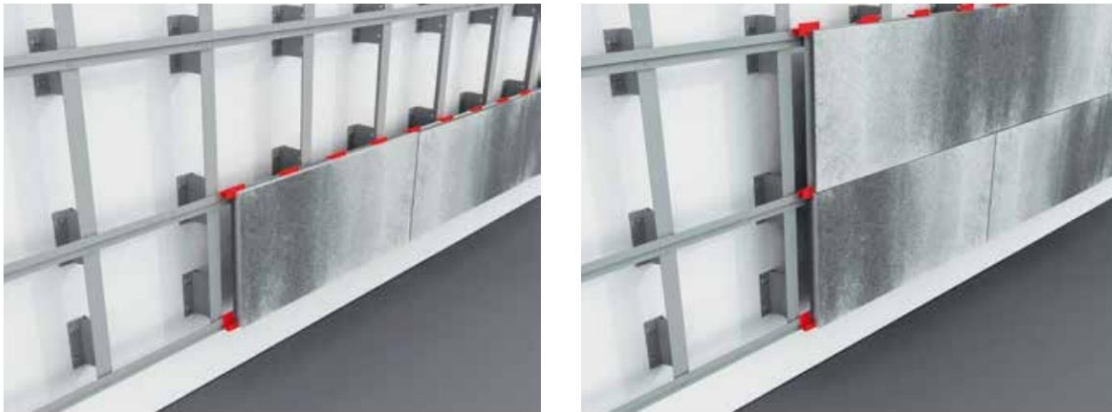
Figure 152: Example of a support grid for unified panels placed on a façade
