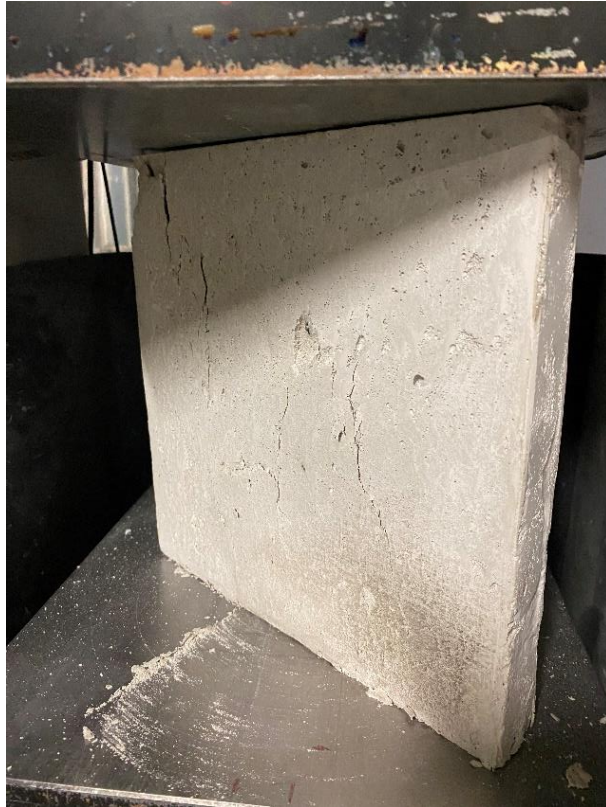
Figure 86: Compressive Strength Test – Solid slab with GF
