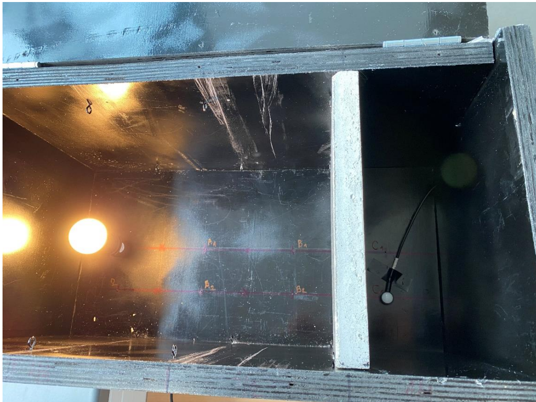
Figure 71: Down-scaled model, points of measurement, artificial light source, sensor
