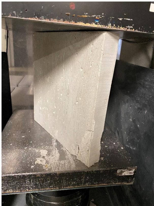
Figure 83: Compressive Strength Test – Solid slab with GF
