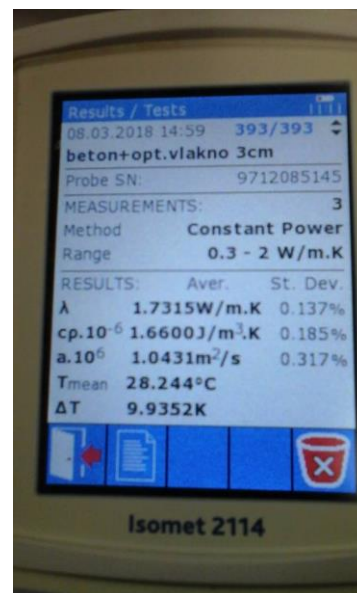
Figure 145: The results of measuring the thermal insulation parameter – Slab with optical fibers 30 m
