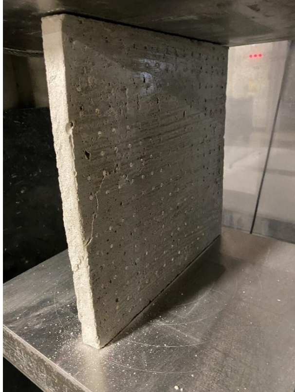
Figure 94: Compressive Strength Test – Slab with POF and GF
