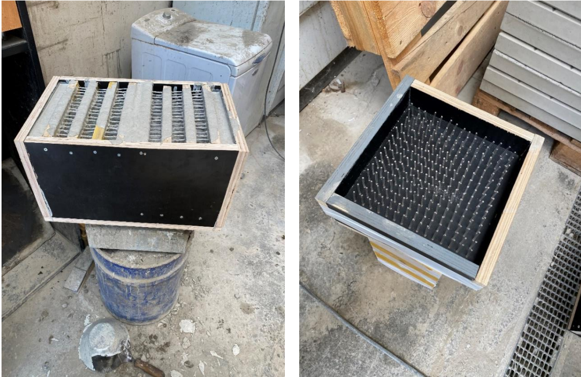
Figure 57: Formworks for making samples
