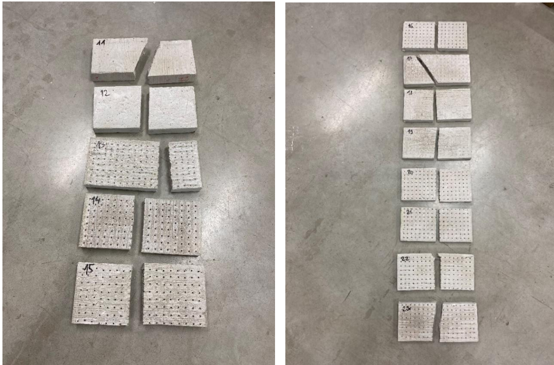
Figure 140: Broken samples after tensile flexural strength test
