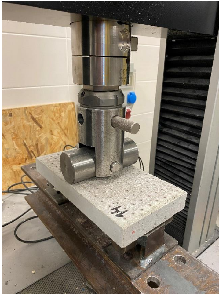
Figure 115: Tensile Flexural Strength Test - Slab with Air holes and GF – Sample 14
