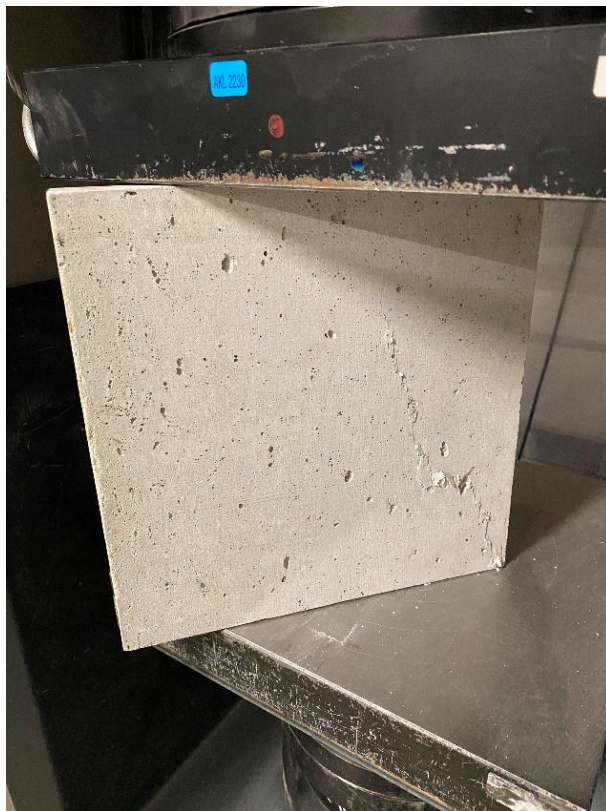
Figure 91: Compressive Strength Test – Solid slab with GF
