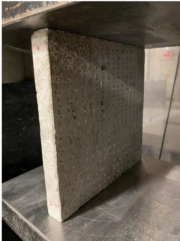
Figure 95: Compressive Strength Test – Slab with POF and GF
