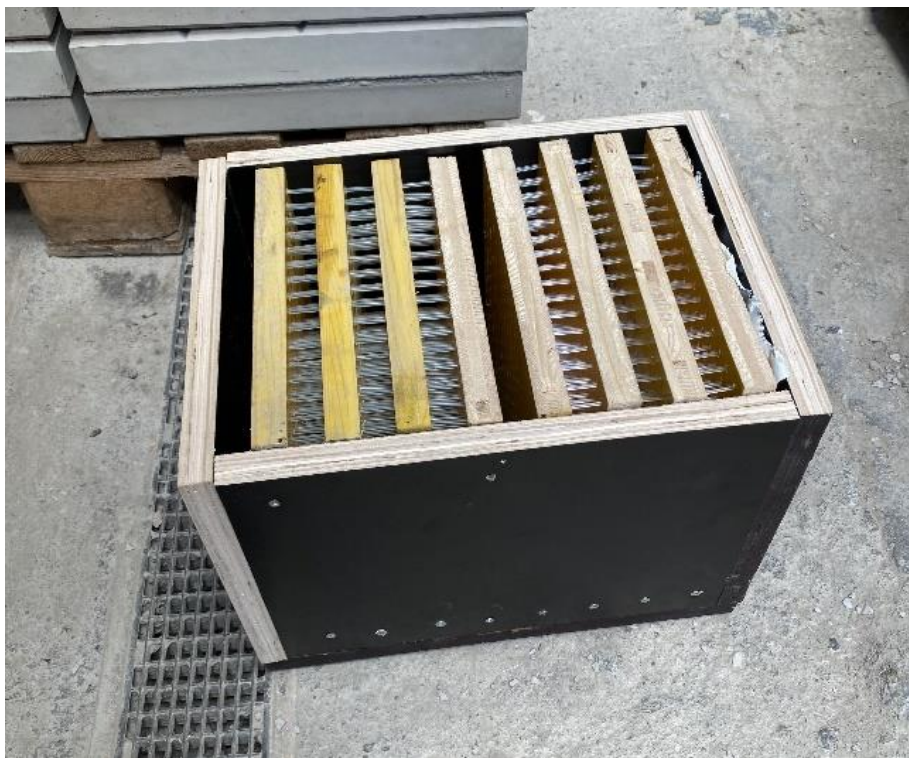
Figure 50: Formworks for making samples
