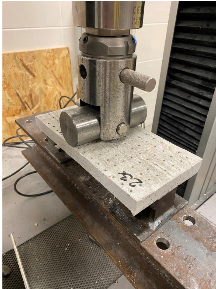
Figure 133: Tensile Flexural Strength Test - Slab with Air holes and GF – Sample 23
