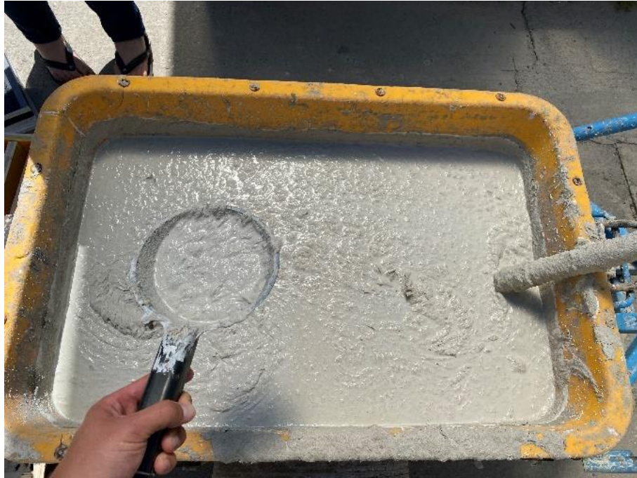
Figure 37: Concrete mixture for samples
