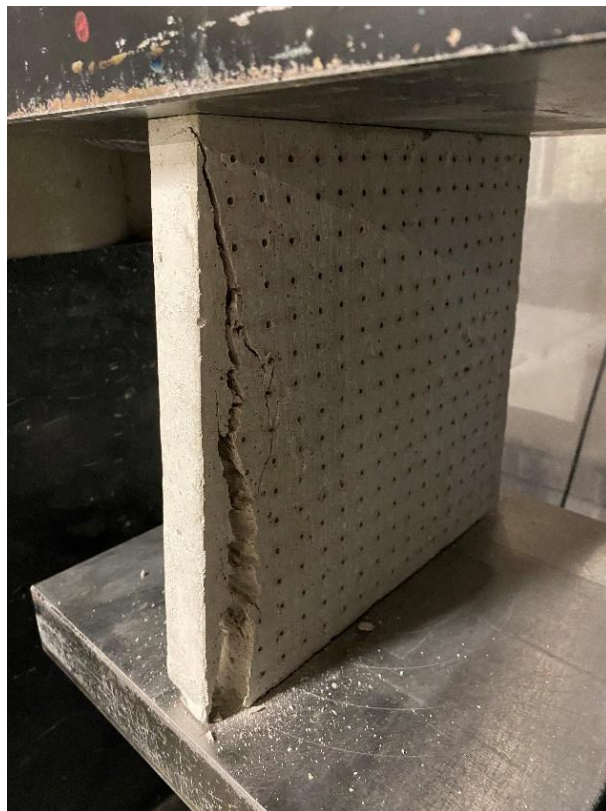
Figure 89: Compressive Strength Test – Slab with Air holes and GF
