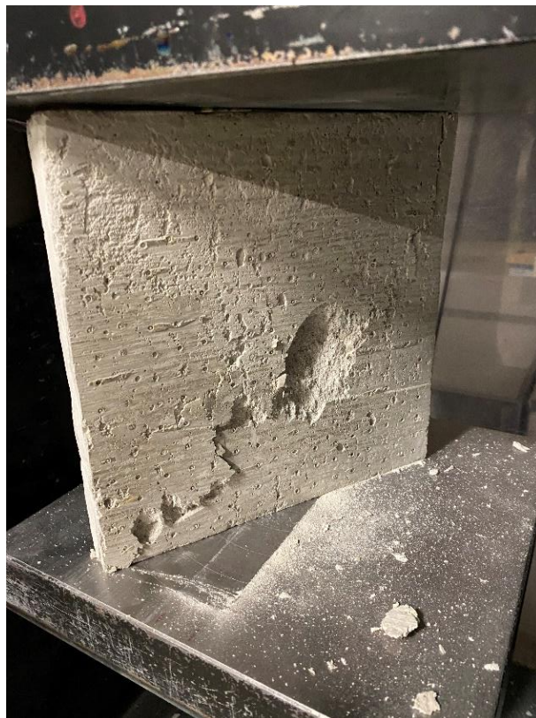
Figure 85: Compressive Strength Test – Solid slab with GF
