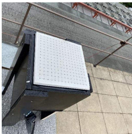
Figure 65: LTC slab on top of the Down-scaled model ready for measuring
