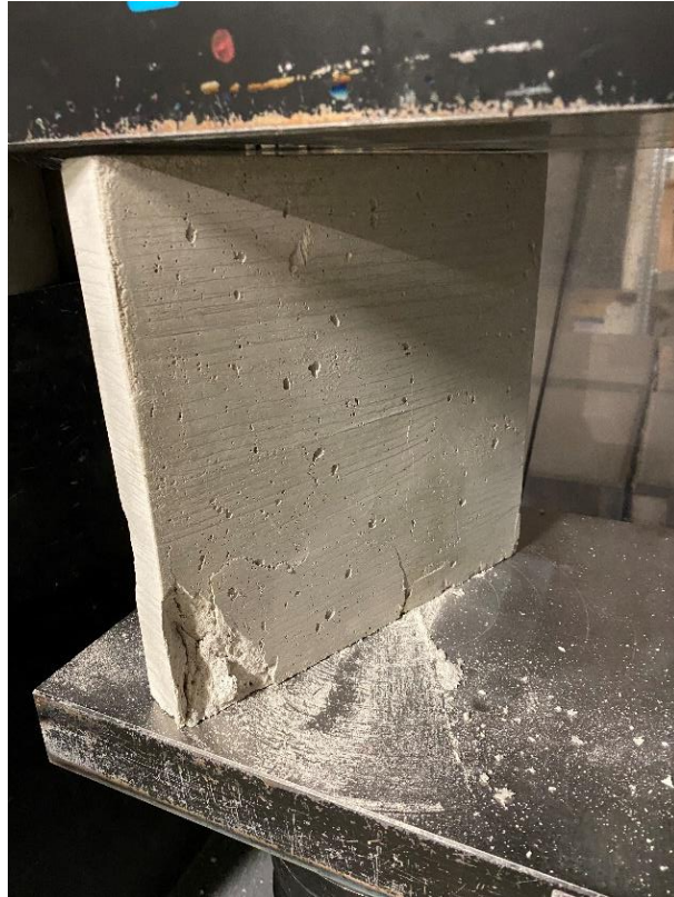
Figure 84: Compressive Strength Test – Solid slab with GF
