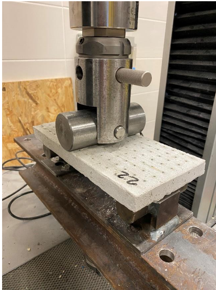
Figure 131: Tensile Flexural Strength Test - Slab with Air holes and GF – Sample 22
