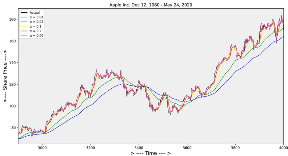
■ Figure 2.3 Simple exponential smoothing with different values of alpha. Figure taken from [35].
