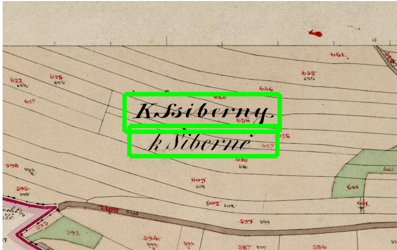
■ Figure 7.11 The output of the finetuned model shows an example where a single ground truth area is detected with multiple smaller detections instead of a single large one.
