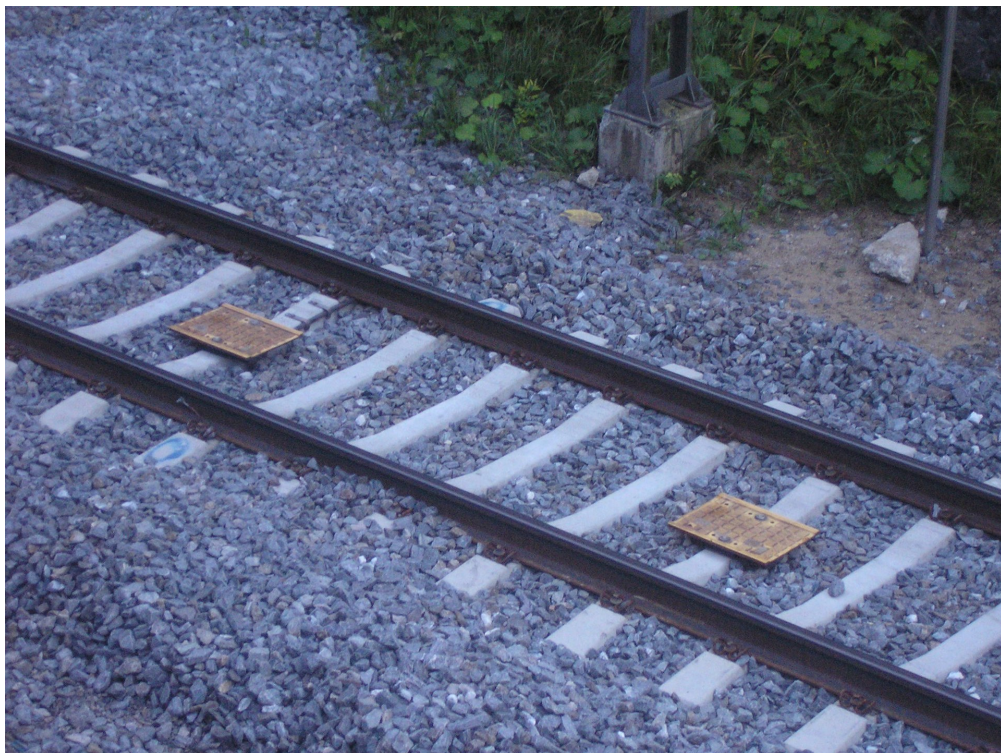
■ Figure 2.2 Balises on Orivesi-Jyväskylä railway in Muurame, Finland (Leppänen 2009). Sourced from [5]
