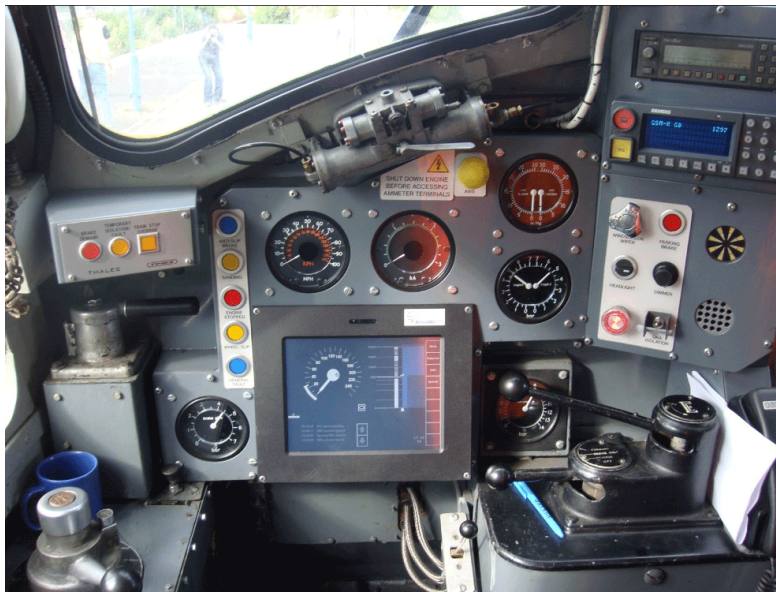
■ Figure 2.4 An example of the DMI inside a train operator cabin. Sourced from [7]
