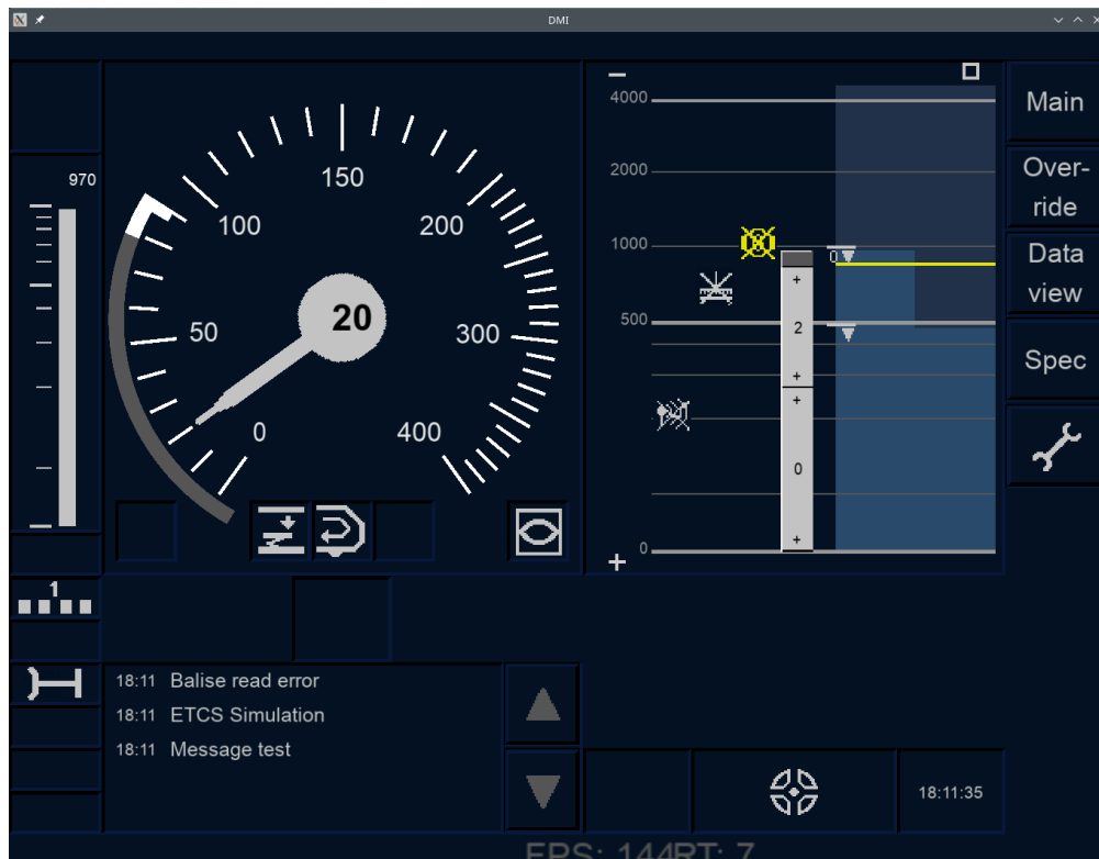
■ Figure 3.8 A screenshot of the DMI display application with the planning area shown.
