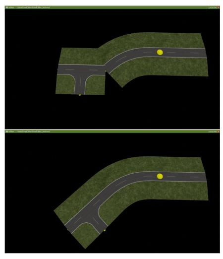
**Figure 5.10:** Smart fitting feature, Top - feature is off in the GUI, Bottom - feature is on; T-cross block being inserted.
