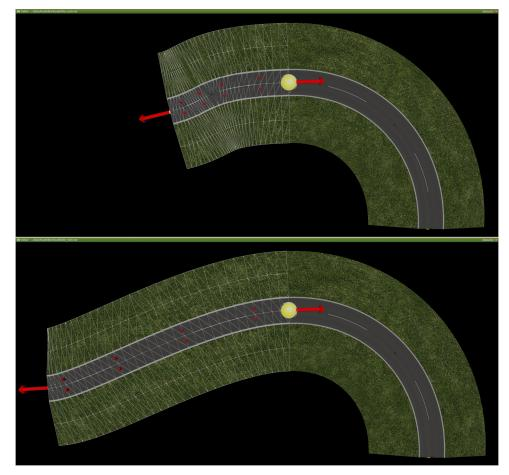
**Figure 5.17:** Comparison of  $C^1$  (top) and  $C^2$  (bottom) Bézier continuity.
