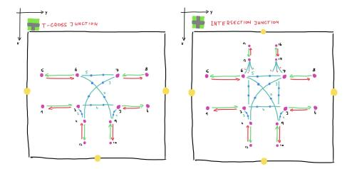
**Figure 5.6:** Traffic block template layout; nodes, forward/backward edges and junctions; Left - T-cross block, Right - intersection block.
