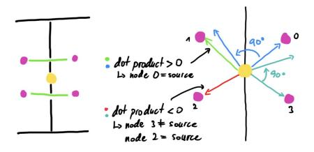
Figure 5.20: Interconnecting lane direction definition description.
