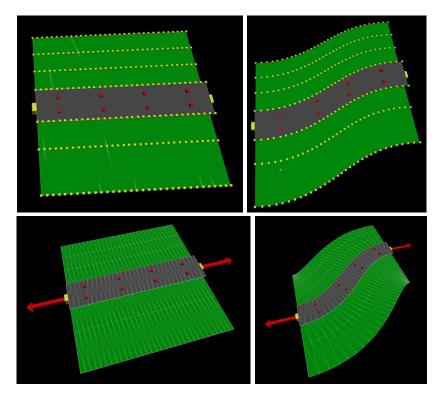
**Figure 5.13:** Block deformations; the first row with only the offset applied, the second row with the curve normal vector applied.
