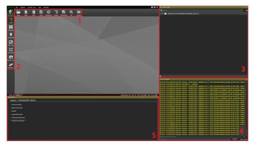
**Figure 3.3:** VRUT - user interface description; 1 - basic scene operation commands; 2 - available modules; 3 - scene graph module; 4 - LOG & Console; 5 - kernel parameters.
