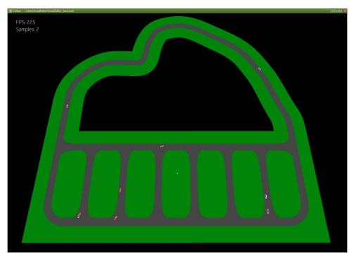
In Figure 6.7 are initial default blocks with a short section created from deformed straight blocks also using *fitting normals* feature and magnetic feature while repositioning connection point to make the road continuous.
