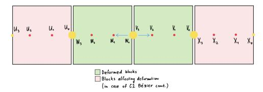
**Figure 5.18:** Blocks' Bézier curve based deformation (each block defined by a 4 control point Bézier curve).
