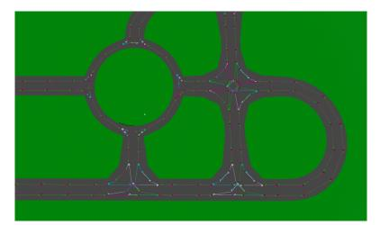
Figure 5.21: Generated road graph with block's traffic interconnections.
