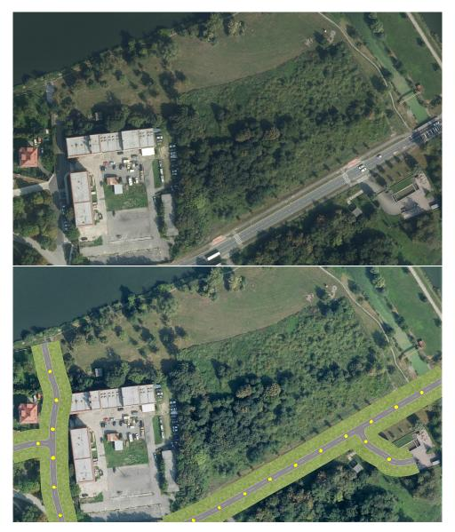
**Figure 6.9:** Scene creation using map background; Top - mere map background; Bottom - traffic network composed using RoadEditor module along the map background's roads.
