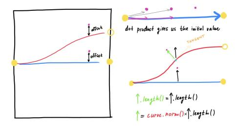
**Figure 5.12:** Vertex reposition based on the curve formation approach description.
