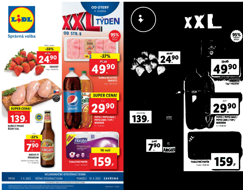
Figure 3.1: OCR Preprocessing - on the left is the original image, on the right is the image after masking just red color (flyer source: www.lidl.cz )
