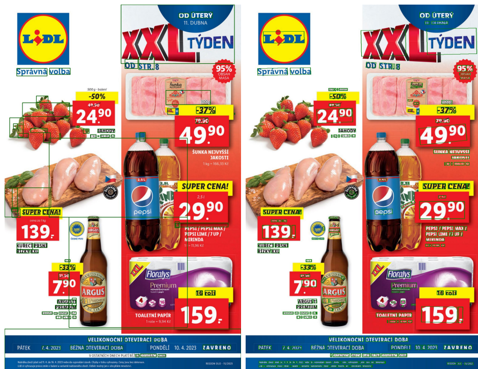
Figure 3.3: Comparison of text areas detected by Tesseract OCR [15] (left) the ones detected with Google Cloud Vision API OCR [12] (right) (flyer source: www.lidl.cz )
