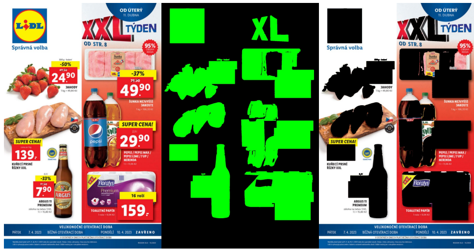
Figure 3.7: Product image detection, from the left to right - a) original image, b) detected product images, c) both images combined (flyer source: www.lidl.cz )
