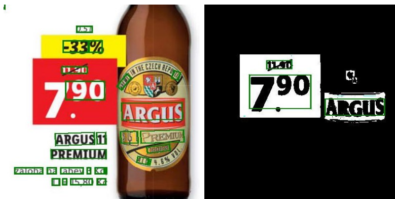
Figure 3.2: Effect of OCR Preprocessing - it is clearer for the OCR that the number 7 is a text after preprocessing (right figure), green bounding boxes show detected text areas (flyer source: www.lidl.cz )
