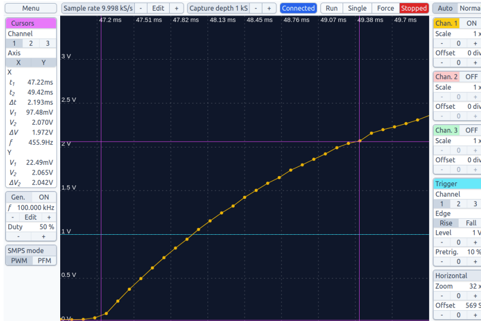
Figure 19: Rising edge of a 100kHz signal captured using ETS.
