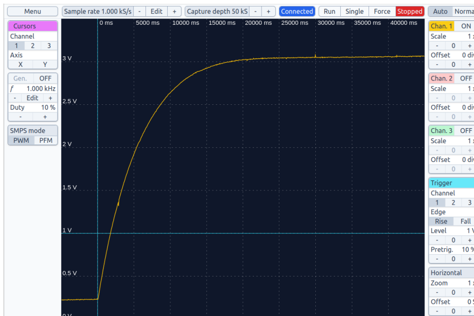
Figure 20: Capture of an 470uF capacitor being charged using Force mode.
