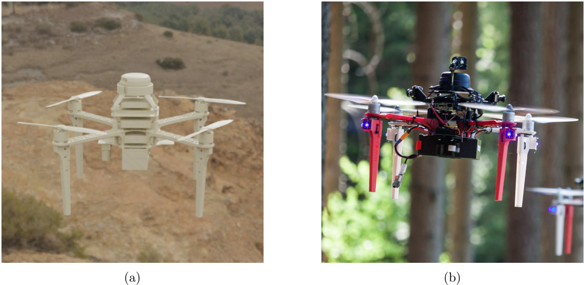
Figure 3.1: Comparison of synthetic (a) and real (b) images of the DJI f450 platform [49] used in this thesis.
