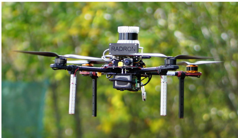
Figure 1.1: A small T650 multi-rotor UAV equipped with the MiniPIX3 sensor. Source: [2].
