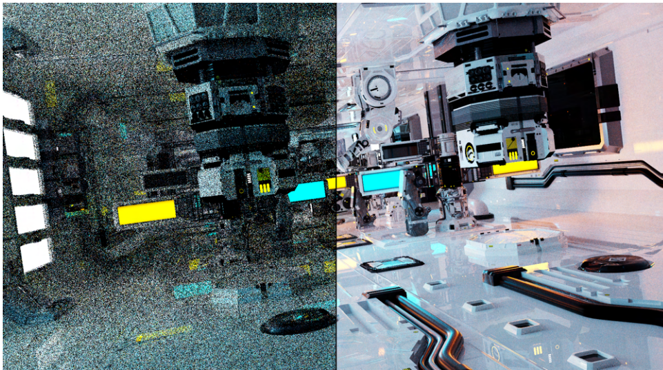
Figure 1.1 : BEEPLE Zero-Day [Win19] scene rendered with path tracing in the Falcor rendering framework [KCK + 22]. (Left) Rendered with path tracing with 1 sample per pixel. (Right) Rendered with path tracing with 1000 samples per pixel.
