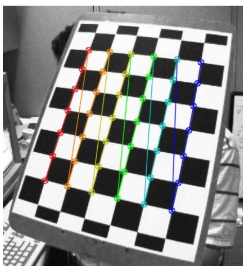
Figure 2.6: Chess calibration pattern. Taken from the OpenCV on-line documentation [54].
