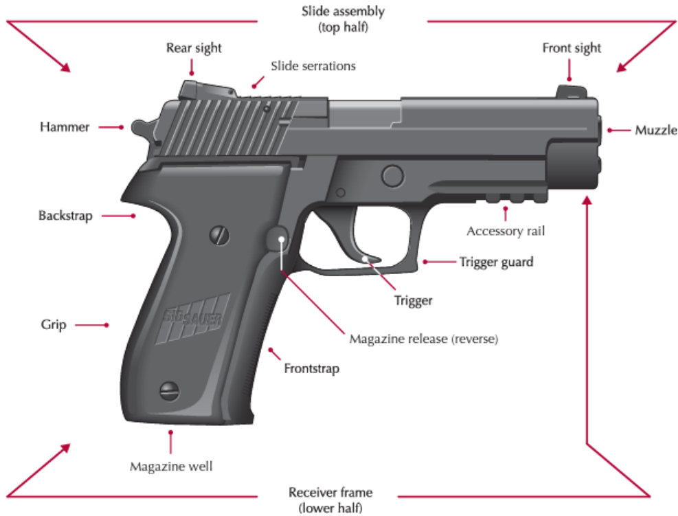
Fig 5: The components of a gun [5]
