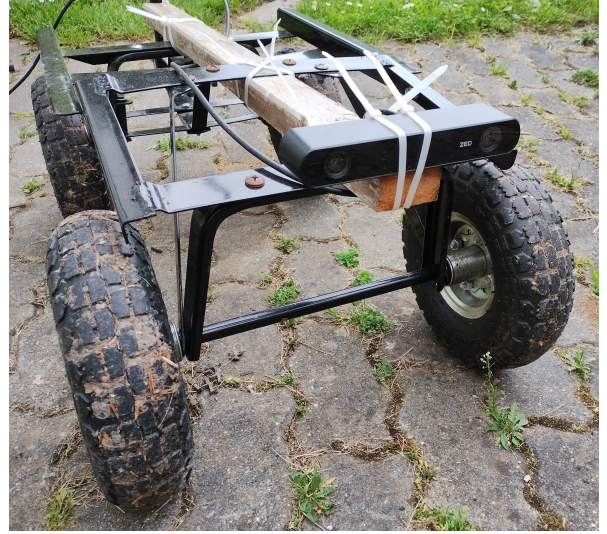
(b) The detail of the ZED 2i stereo camera
