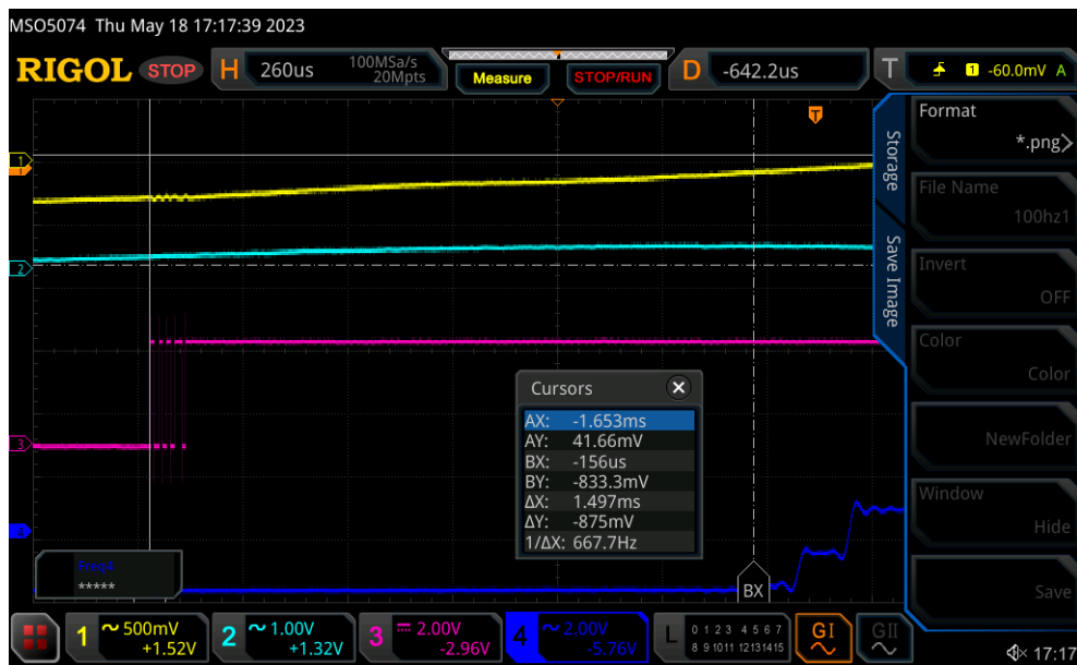
Figure 5.10: 8kHz Sampling Rate 100 Hz Sinewave Modulation Close Up - microphone output (yellow curves), acoustic pressure input (aqua curves), Sigma-Delta output (magenta curves), demodulated signal (blue curves)
