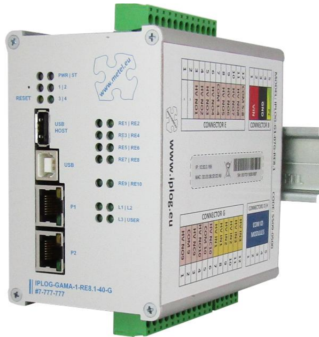
Figure 4.1: An industrial PLC from the contractor’s IPLOG-GAMA series using the same aluminium chassis as the intended product
