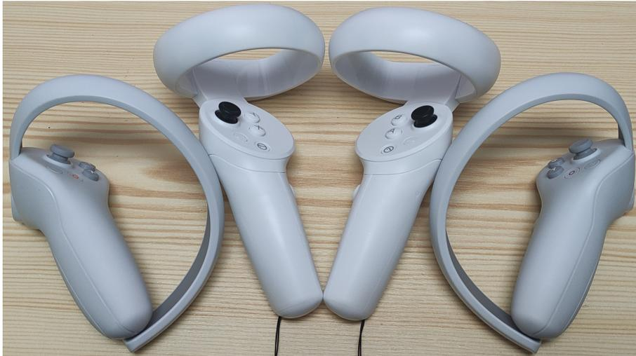
**Figure 5.1.** Photo of controllers used with PICO headsets. PICO 4 controllers are to the side and Pico Neo 3 controllers are in the middle.
