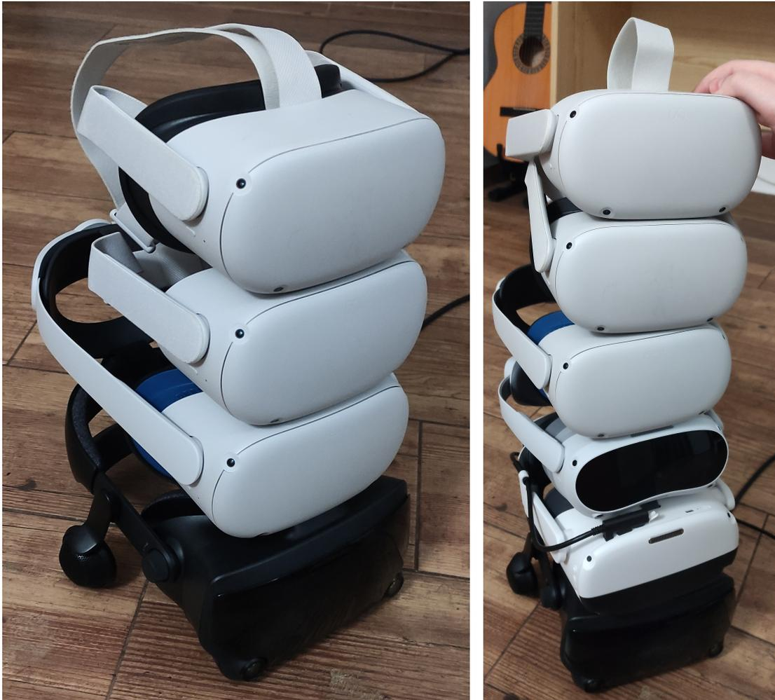
**Figure 3.3.** Stack of headsets used for tower of doom method. Demonstrates how the method works in practice and also shows that while possible to use, the method does not scale well beyond four headsets (at least for those particular models).
