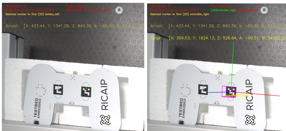
Figure 6.1: Visualization of adding a never-seen-before part
