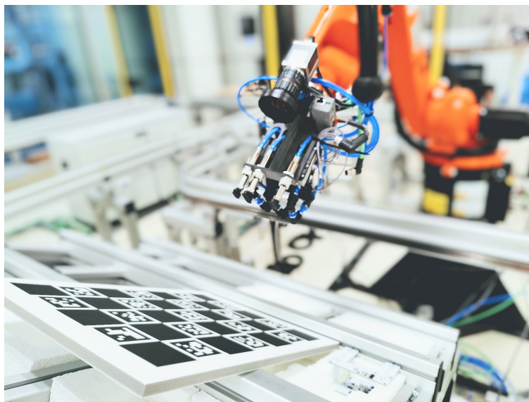
Figure 5.8: CharUco pattern developed on a rigid board
