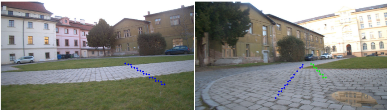
Figure 4.12: Two selected images with very incorrect detections of lane borders. All detected lane borders face the forward direction.
