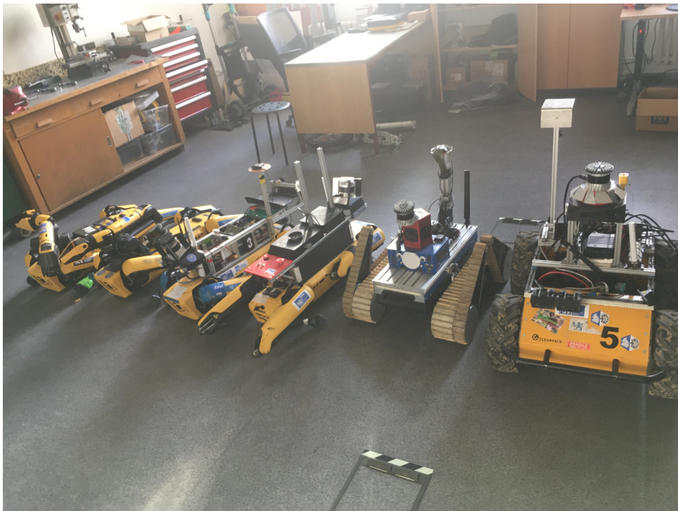
Figure 3.1: Robot fleet, from the left: 2x Spot with arm, 2x Spot without arm, TRADR, Husky
