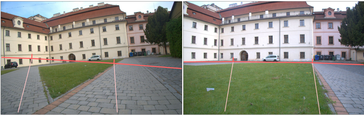
Figure 4.15: Left: Rendered horizon and heading lines do not line up with the image – the transformation used and the photo itself are each from a different time; Right: Rendered horizon and heading lines are in sync with the picture.
