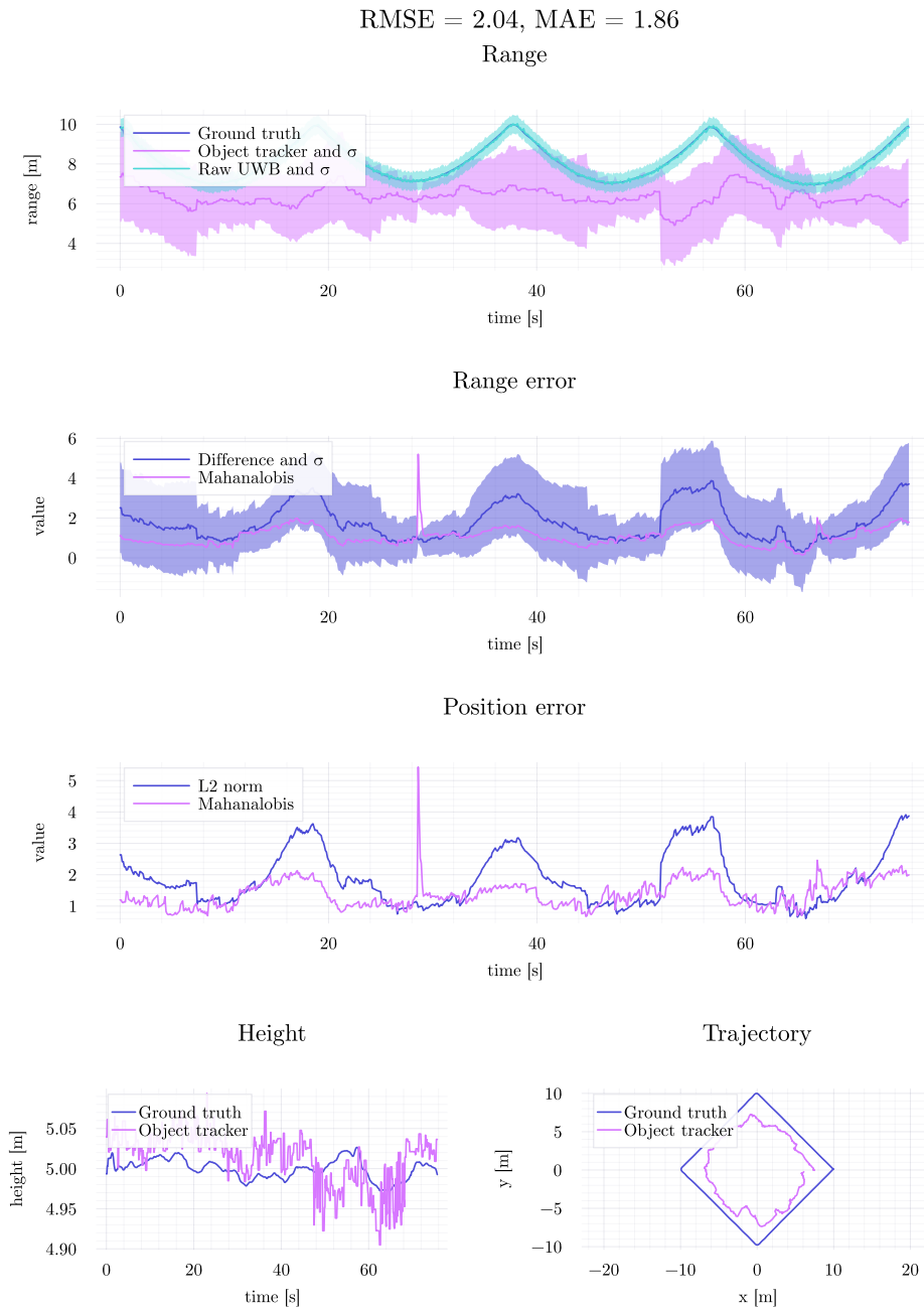
Figure C.5: Square path with UWB fusion.
