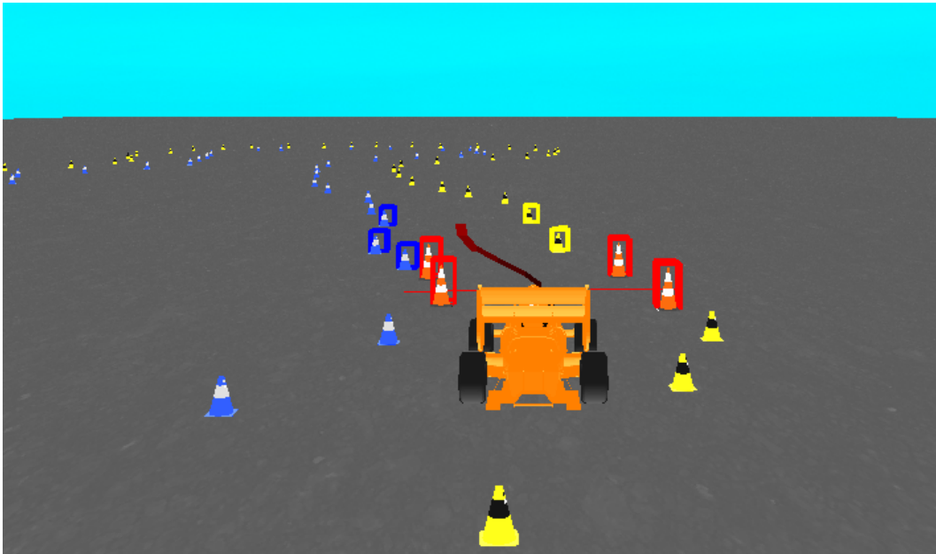
Figure 3.5: Illustration of the path planning test performed in the simulator 3.2 on Autocross 2 track 3.1. The car is situated at the starting position and begins its motion. Detected cones are visually represented by 3D bounding boxes, and the planned path is shown as a dark red line.
