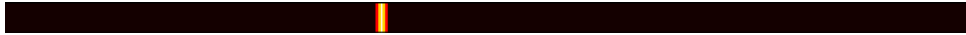
Figure 3.5: One dimensional ground-truth heatmap for the left boundary of the track representing the confidence of pixels being on the position of left boundary of the race track
