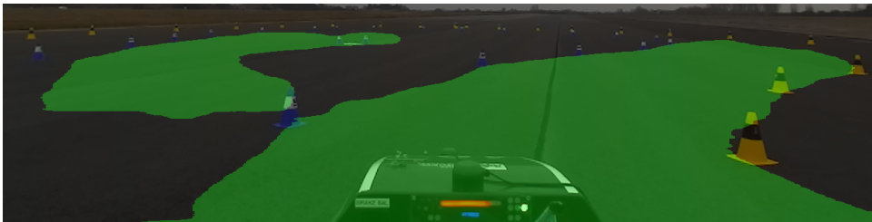
Figure 3.3: Segmented race track with mispredicted pixels in the left part
