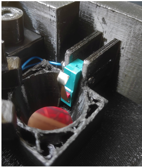
Figure 2.10: Modified electromechanical switch
