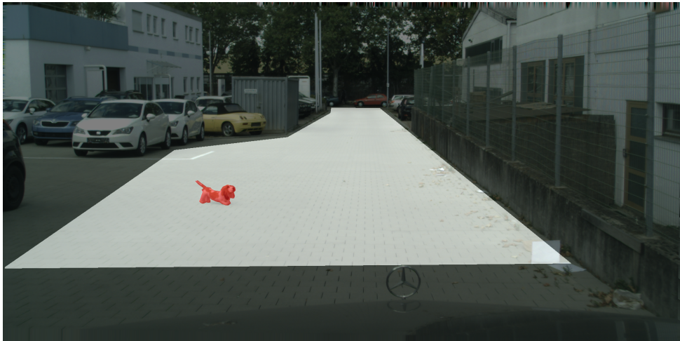
Figure 3.1: Image from the LostAndFound dataset [11]. The region of interest is highlighted in white, with the anomalous object highlighted in red.
