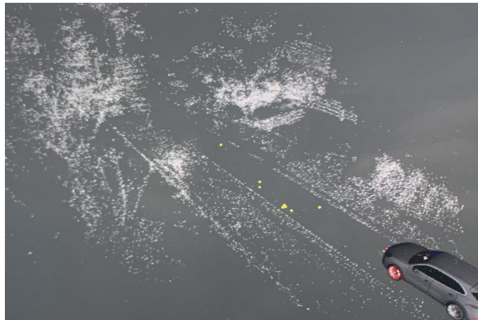
Figure 3.14: An example of visualization of a LiDAR scan with very few points in front of the vehicle.
