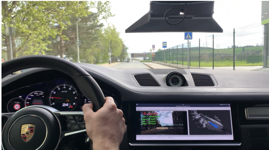
Figure 4.5: Speed limited by detecting speed bump by the LiDAR detector.
