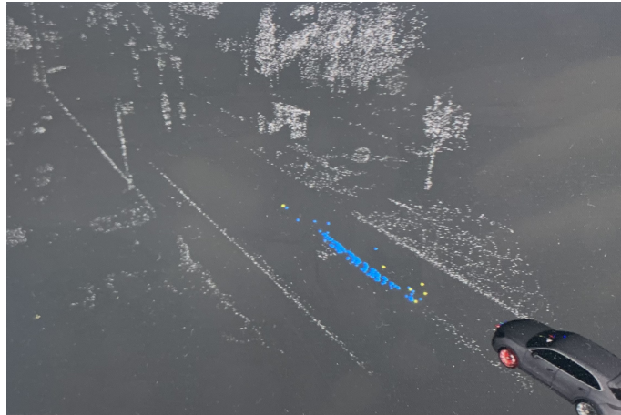
Figure 3.13: An example of visualization of a LiDAR scan with a missing road plane in rainy weather.
