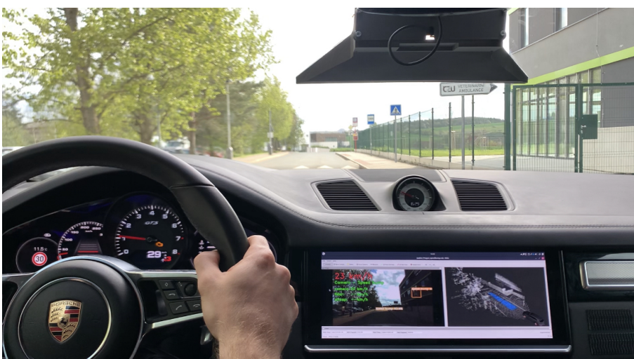
Figure 4.4: Speed limited by detecting speed bump by the camera detector.
