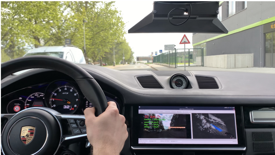
Figure 4.3: Speed limited by detecting speed bump warning sign by the camera detector.
