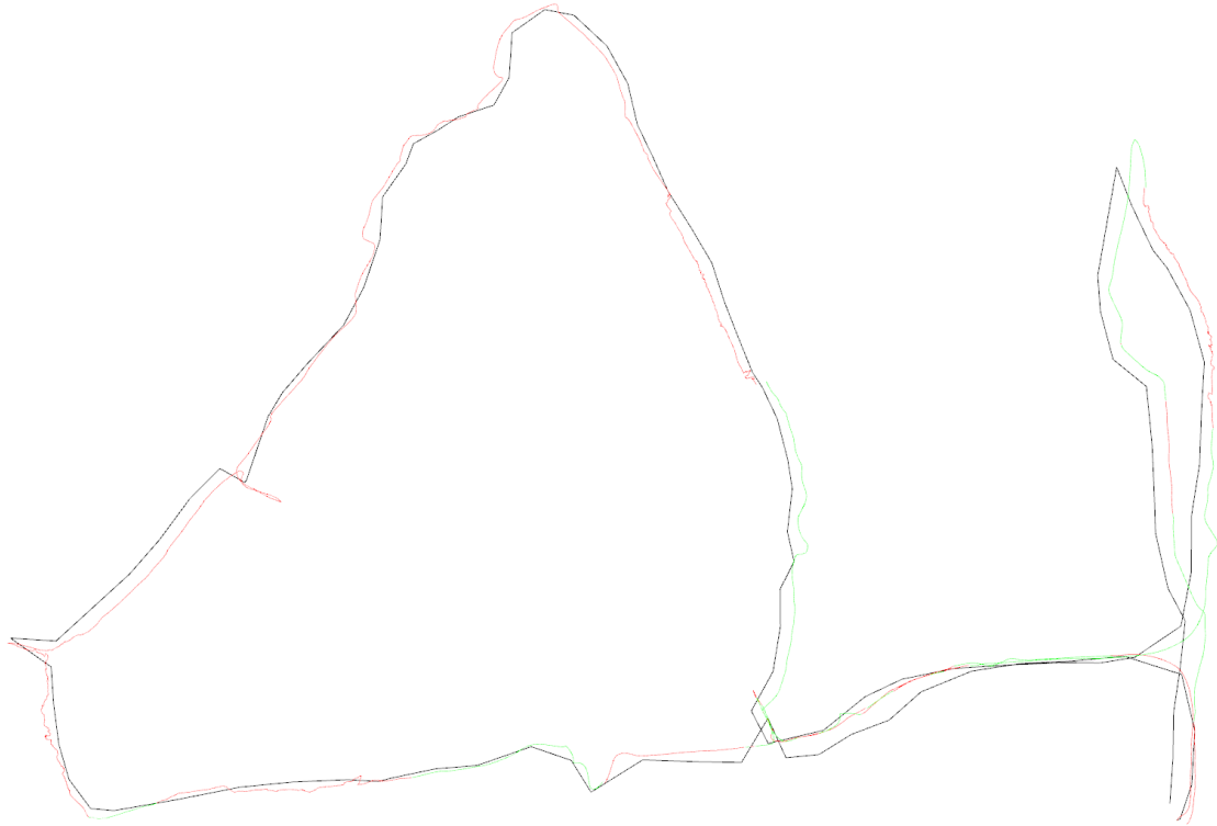
Figure 6.7: A comparison of the estimated pose from GPS by Voxgraph factor graph (black) compared to RTK GPS (green and red).
